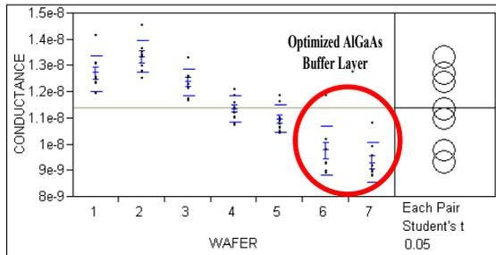
Figure 7: Conductance (1/Resistance) of the collector isolation structure from MESFET epi. Wafers with the optimized AlGaAs buffer layer are highlighted in circle.
