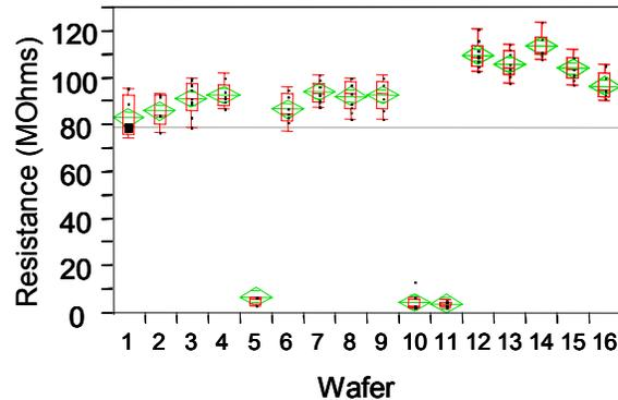
Figure 4: Collector isolation resistance as a function of experimental conditions given in Table 1.
