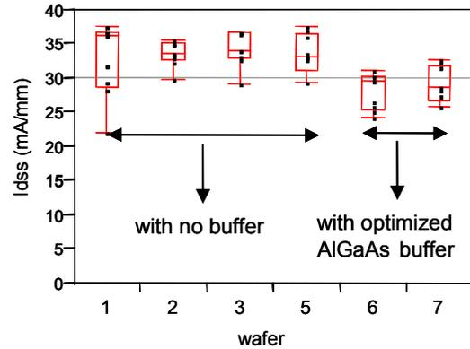
Figure 9: Saturation current ( $I_{dss}$ ) in mA/mm of the 1x100  $\mu\text{m}$  epi MESFET device. No statistical difference is observed between the epi wafers with or with no buffer layer.
