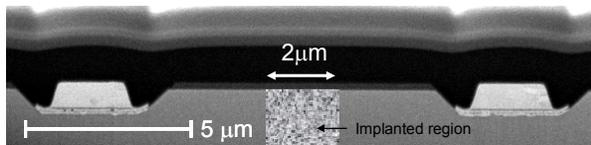
Figure 3: SEM cross-section of the collector isolation structure with the shaded implanted
