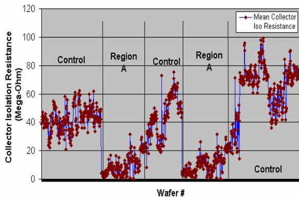
Figure 1: Collector Isolation Resistance Trend
