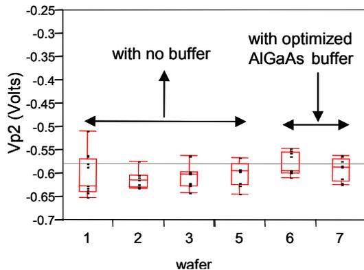
Figure 8: Pinch off voltage of 1x100  $\mu\text{m}$  epi MESFET device. There is no influence of AlGaAs buffer on the FET parameters.
