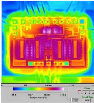
Figure 6: Thermal profile of open cavity PAM with AlGaAs buffer
