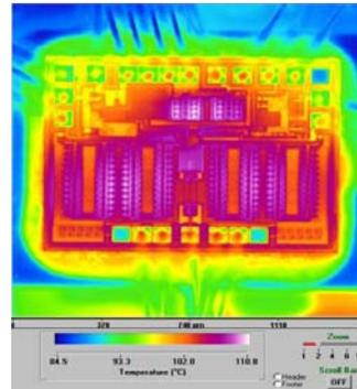
Figure 5: Thermal profile of open cavity PAM with no buffer
