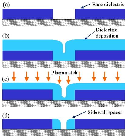
Figure 1: Schematic of sidewall spacer concept
