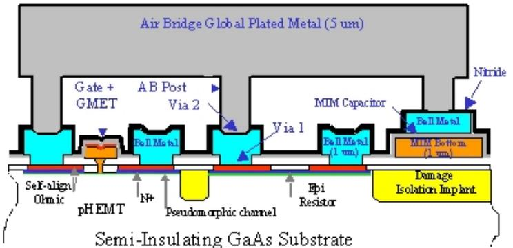
Figure 3: Schematic cross-section of the TQP13 process
