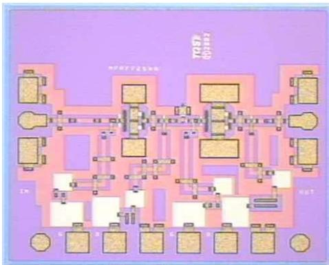
Figure 8: Photo of 77 GHz 2-stage Medium Power Amplifier.
