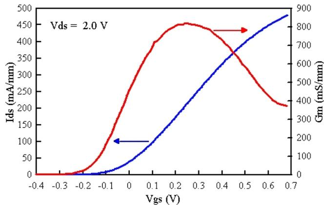
Figure 5: Transfer characteristics ( $I_{ds}$  and  $G_m$  vs.  $V_{gs}$ ).
