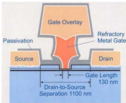
Figure 2: Schematic of TQP13 transistor.
