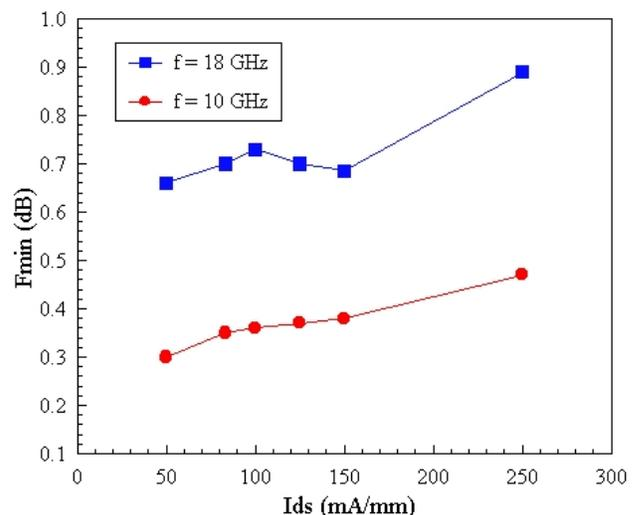
Figure 7: Noise figure as a function of drain current at frequencies of 10 and 18 GHz.
