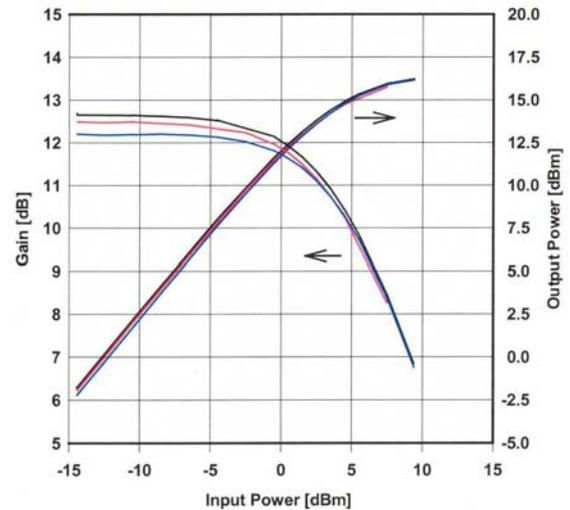
Figure 9: Gain and Pout of 77 GHz 2-Stage Medium Power Amplifier for automotive radar applications.
