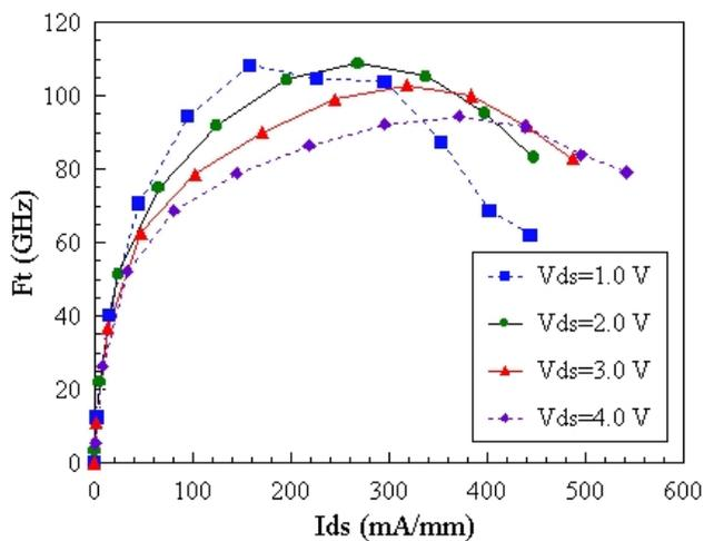
Figure 6:  $F_t$  as a function of  $I_{ds}$  for a nominal TQP13 device.
