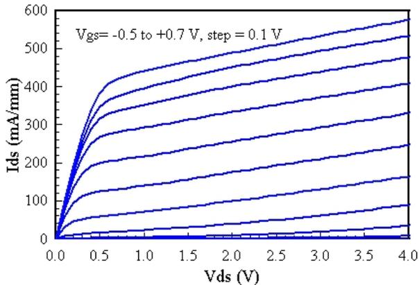
Figure 4:  $I_{ds}$  vs.  $V_{ds}$  relationship.
