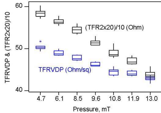
Figure 3. Quartile plot of NiCr deposition pressure effect on the difference between NiCr sheet resistance (TFRVDP) and one tenth of the narrow resistor resistance (TFR2x20).
