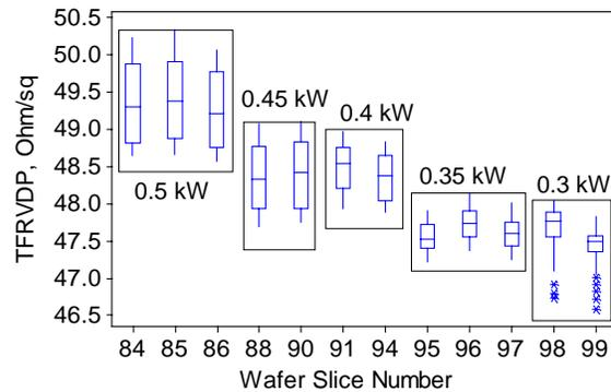
Figure 4. Effect of NiCr target power on NiCr uniformity.
