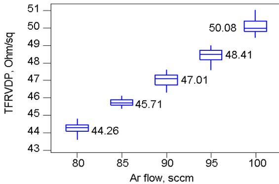
Figure 5. Effect of Ar flow rate on NiCr sheet resistance.
