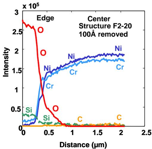
Figure 2. Auger Analysis indicated that the NiCr edge had higher oxygen content.
