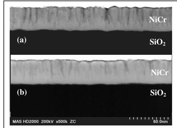
Figure 6. NiCr film on SiO<sub>2</sub> dielectric. (a) SiO<sub>2</sub> film was processed right after chamber showerhead change. (b) SiO<sub>2</sub> film was processed after normal conditioning.
