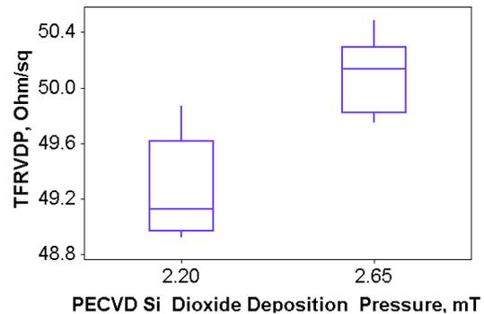
Figure 7. Effect of Si dioxide deposition pressures on NiCr sheet resistance. Eight wafers were processed at each deposition pressure.
