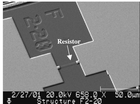
Figure 1. TriQuint  $2 \mu\text{m} \times 20 \mu\text{m}$  resistor.
