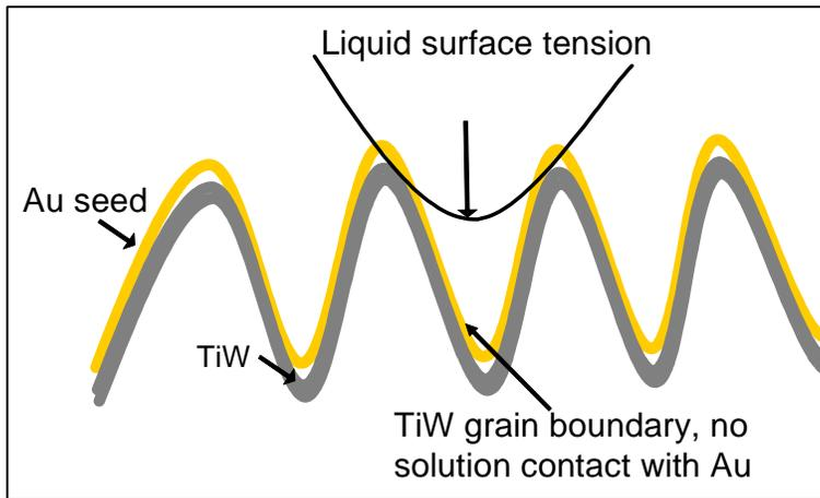
Figure 5: Representation of incomplete reverse plating
