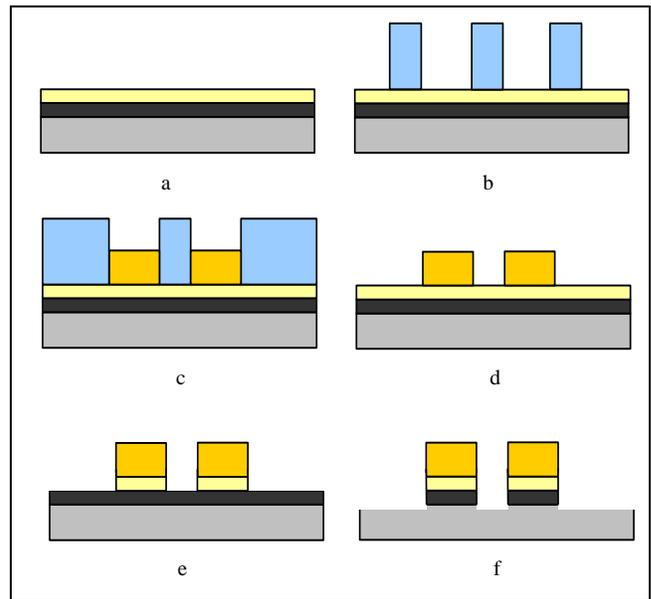
Figure 1: Representation of individual processing steps in formation of patterned, electroplated, metal features.
