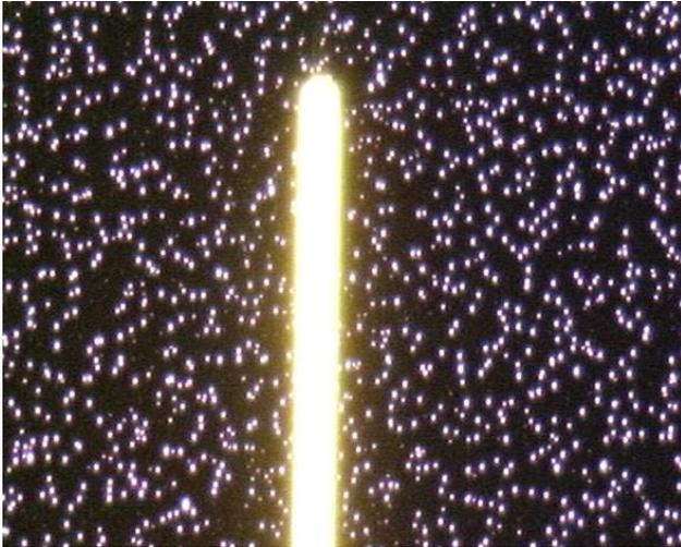
Figure 2: Dark field image of defects. Highlighted bar in center is a plated metal feature.
