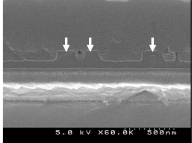
Figure 4: SEM cross-section. Arrows indicate mesa defects in dielectric layer.
