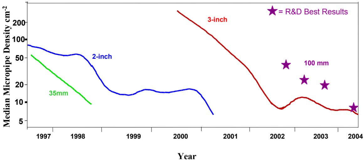
Figure 1: Progress in reduction of Cree’s median micropipe density in production n-type 4H-SiC versus time. Also included are “R&D Best” results on 100 mm wafers.
