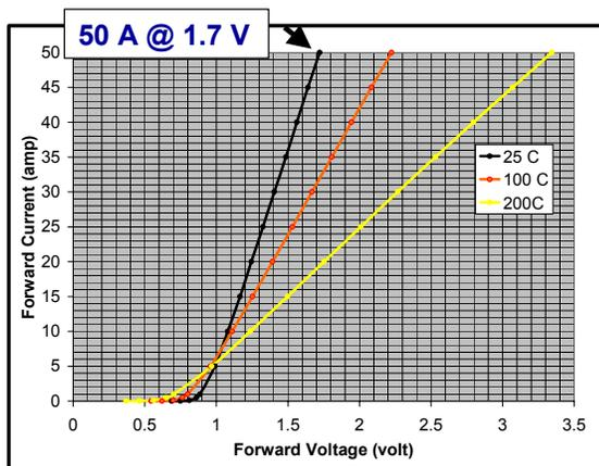
Figure 2: Forward I-V characteristics of the 1200 V, 50 A SiC Schottky diode, with a chip size of 5.6mm x 5.6 mm.
