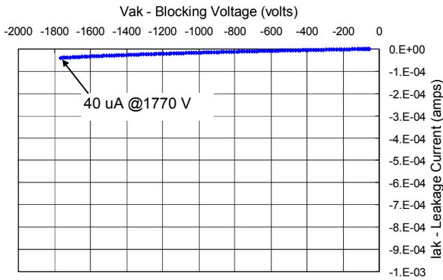
Figure 8: Forward blocking voltage of a 1 cm<sup>2</sup> 4H-SiC thyristor device.
