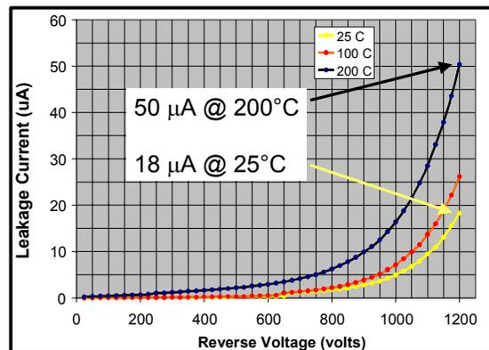
Figure 3: Reverse I-V characteristics of the 1200 V SiC Schottky diode at room temperature, 100°C, and 200°C.
