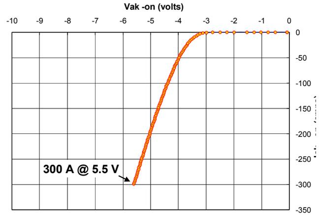
Figure 9: The forward I-V characteristics of the 1 cm<sup>2</sup> thyristor at room temperature. A gate current of 100 mA was used.
