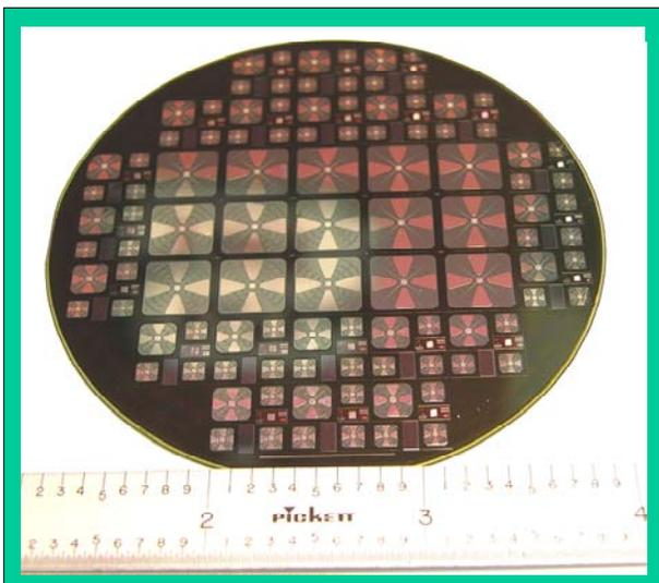
Figure 6: Picture of a 3 inch SiC wafer with fifteen 1 cm<sup>2</sup>, and many smaller, thyristors.
