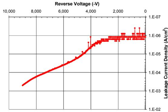
Figure 4: Reverse J-V characteristic of a 50 A diode (8.7 mm x 8.7 mm) showing >9 kV blocking (solid curve) that is current compliance limited. The dashed line extrapolates the reverse blocking to 10 kV.
