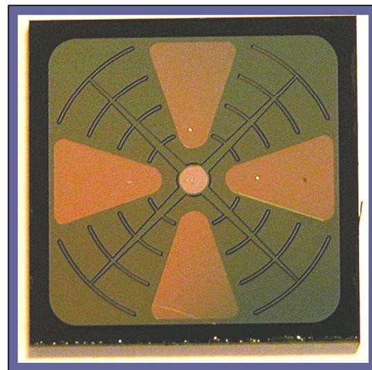
Figure 7: Picture of a 1 cm<sup>2</sup> SiC thyristor chip.
