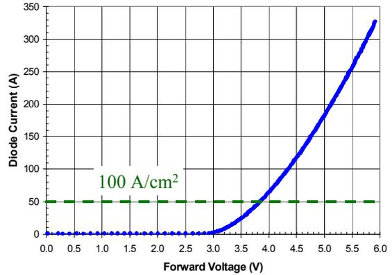
Figure 5: Pulsed forward I-V characteristic of a large 10 kV diode with a 3.9 V forward drop at 50 A and 5.9 V forward drop at 328 A, indicating a high level of conductivity modulation.
