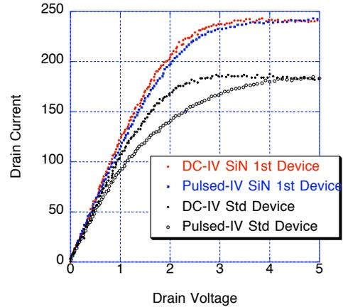
**Figure 2. DC vs pulsed IV for  $\text{Si}_3\text{N}_4$  1st and standard processed devices. Pulsed bias conditions  $V_{\text{ds}} = 20\text{v}$ ,  $V_{\text{gs}} = -7\text{v}$**
