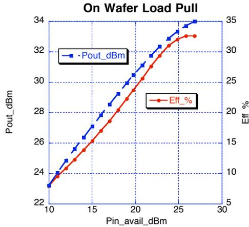
**Figure 4. Pout and efficiency as a function of available input power for silicon nitride 1<sup>st</sup> process.**
