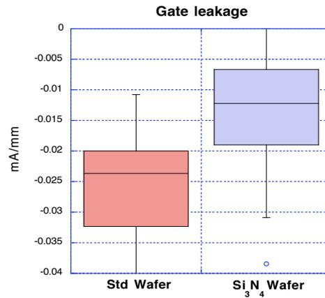
**Figure 3. Boxplots of gate leakage measured on standard and experimental processed wafer**
