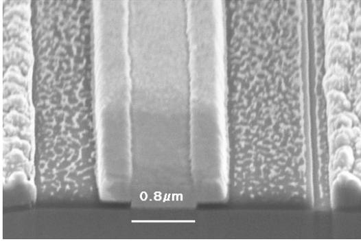
**Figure 1. Silicon Nitride 1st processed gate cross-section**
