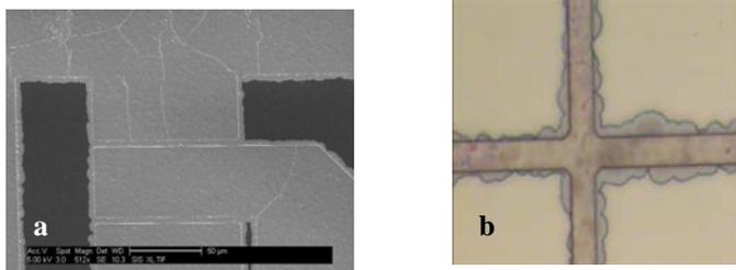
Figure 2 – R.I. 2.2 SiN encapsulation – (a) HEMT micrograph showing crack pattern (SEM); (b) EBAM surrounded by “clouds”.
