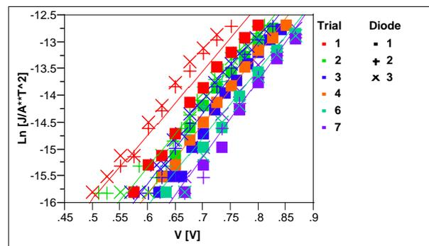
Figure 4 -  $\ln [J/A^{**}T^2]$  as a function of V immediately after diode lift-off.
