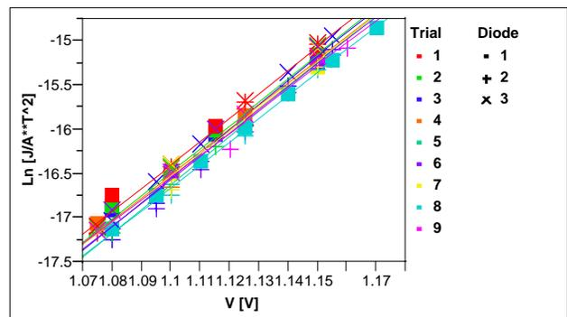
Figure 9 -  $\ln [J/A^{**}T^2]$  as a function of V after annealing at 300°C for 24h.
