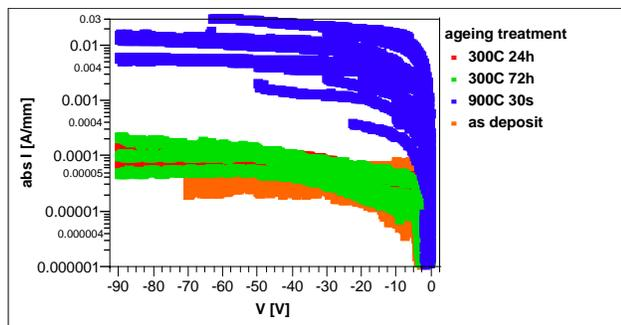
Figure 11. Leakage current as a function of reverse bias after annealing by different treatments.
