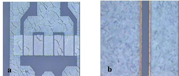
Figure 1 –R.I. 1.79 SiN encapsulation: - (a) HEMT micrograph showing crack pattern (x100); (b) metal morphology and edge definition (x1000).
