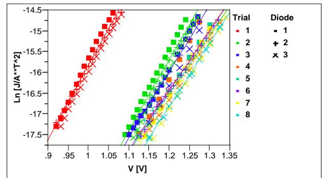
Figure 8 -  $\ln [J/A^{**}T^2]$  as a function of V after diode lift-off.
