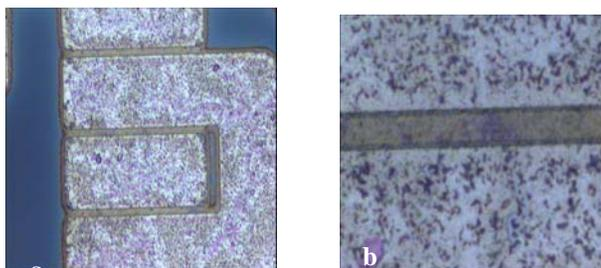
Figure 3 – SiO<sub>2</sub> capping – (a) HEMT micrograph showing no cracks (x200); (b) metal morphology and edge definition surrounded by “clouds” (x1000).
