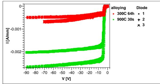
Figure 7 - diode leakage current as a function of the reverse bias after annealing by different treatments.
