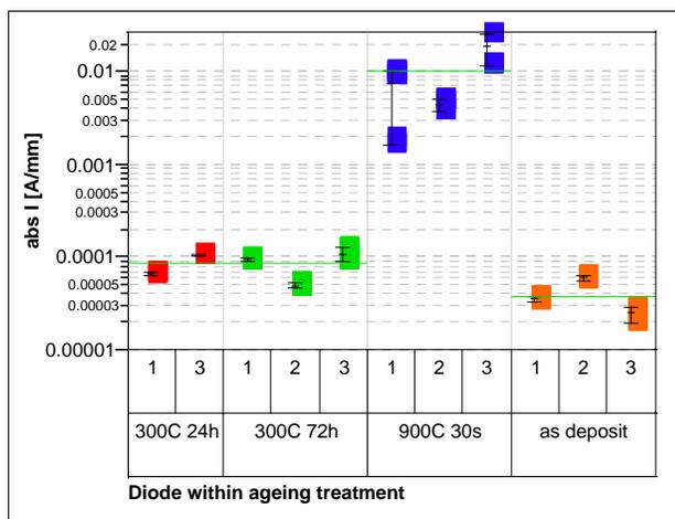
Figure 12. Leakage current at reverse 50V bias after annealing by different treatments.
