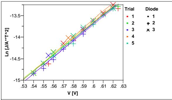
Figure 5 -  $\ln [J/A^{**}T^2]$  as a function of V after annealing at 300°C for 24 h.
