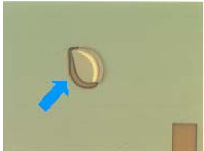
Figure 1. Example of photoresist blister observed on oxygen plasma cleaned silicon nitride surface after UV exposure in the photo stepper.
