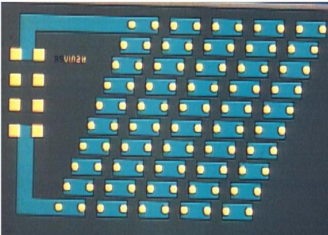
Figure 1: Front side of via chain
