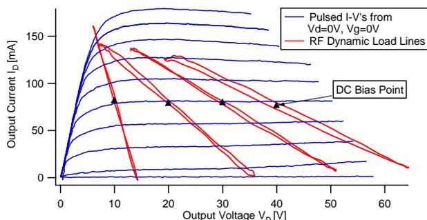
Fig. 2. RF dynamic load-lines at different drain voltage bias points.
