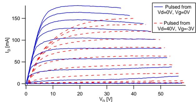
Fig. 1. Pulsed DC I-V measurements.  $V_G$  ranges from -8V  $\rightarrow$  +2V in 1V steps
