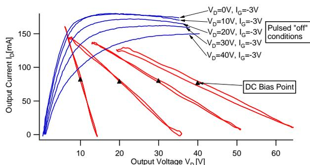
Fig. 4. RF dynamic load-lines superimposed on pulsed DC I-V's pulsed from the same bias points.
