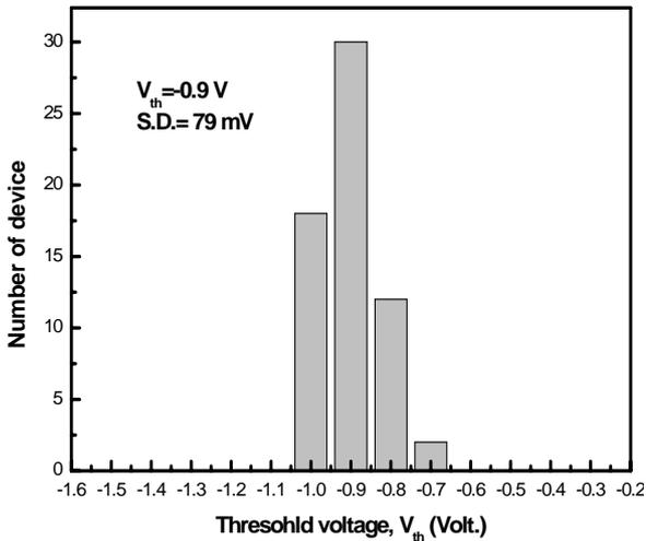
Fig. 2 The histogram of  $V_{th}$  for 0.25- $\mu\text{m}$  gate-length  $\text{In}_{0.5}\text{Al}_{0.5}\text{As}/\text{In}_{0.5}\text{Ga}_{0.5}\text{As}$  metamorphic HEMTs using succinic acid in the gate-recess fabrication.
