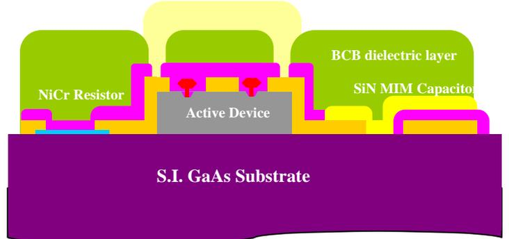
Fig. 3 The cross section of BCB-bridged MMIC process including active device, NiCr resistances, SiN capacitors.
