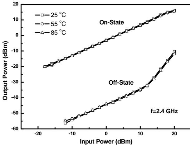
Fig. 7 Measured the on and off states output power versus input power characteristics at 2.4 GHz of SPST switch from 25 °C to 85 °C.
