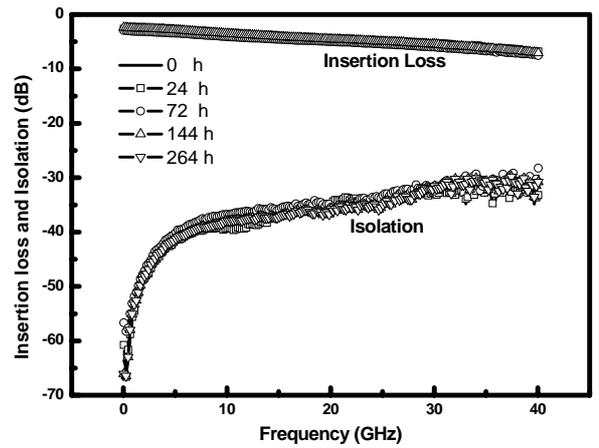
Fig. 6 The insertion loss and isolation of SPST switch measured under an 85-85 environment for 264 hrs.
