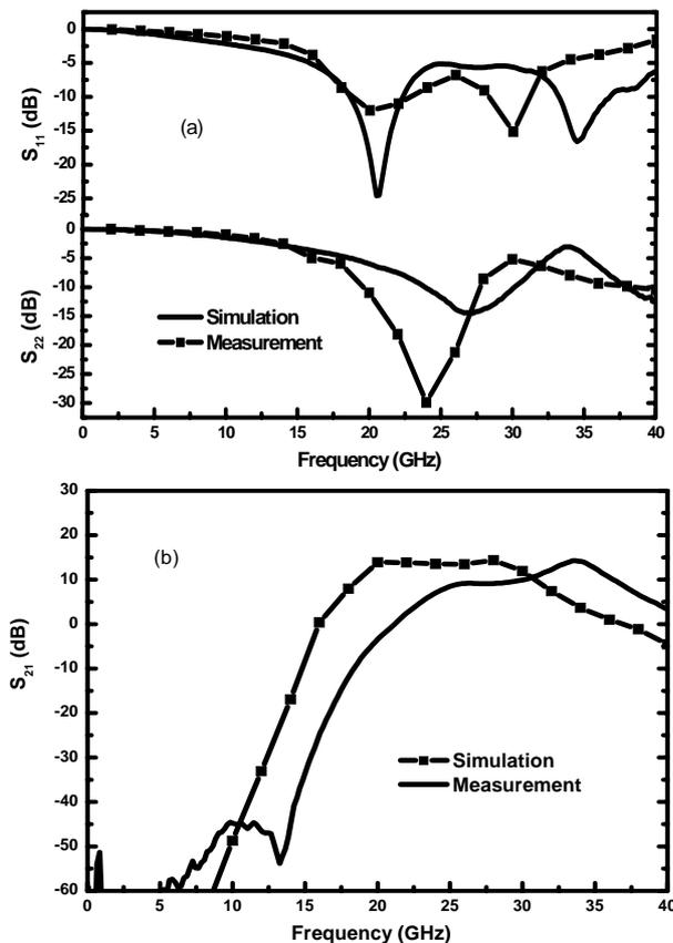
Fig. 4 The simulated and measured results of  $S_{11}$  and  $S_{22}$  (a), and small signal gain,  $S_{21}$  (b).
