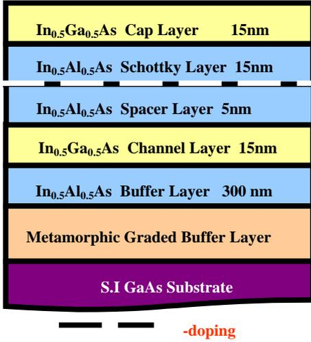
Fig. 1 The device cross-section of the  $\text{In}_{0.5}\text{Al}_{0.5}\text{As}/\text{In}_{0.5}\text{Ga}_{0.5}\text{As}$  metamorphic HEMTs
