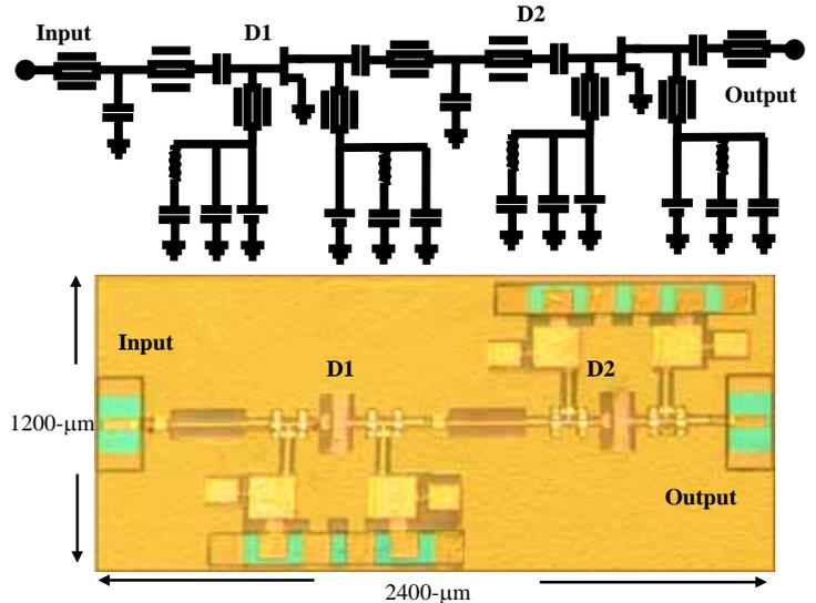
Fig. 3 The schematic circuit topology and the chip photograph for monolithic Ka-band gain amplifier
