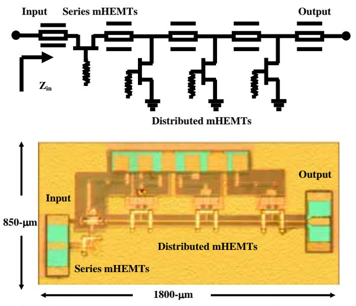
Fig. 5 The schematic circuit topology and the chip photograph for monolithic distributed SPST switch using 0.25- $\mu\text{m}$  T-gate  $\text{In}_{0.5}\text{Al}_{0.5}\text{As}/\text{In}_{0.5}\text{Ga}_{0.5}\text{As}$  mHEMTs.
