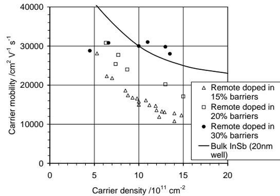
Figure 1. Hall mobility data on Te modulation doped 20 nm thick InSb quantum wells with 15%, 20% and 30% Al in the  $\text{Al}_x\text{In}_{1-x}\text{Sb}$  barrier layer, with the bulk doped equivalent shown for comparison.
