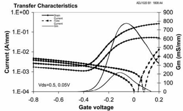
Figure 4.  $0.1 \mu\text{m}$   $L_G$  InSb QW transistor transfer characteristics at  $295 \text{ K}$ ,  $L_{DS} = 1 \mu\text{m}$ ,  $W_G = 40 \mu\text{m}$ ,  $V_{DS} = 0.5 \text{ V}$  and  $0.05 \text{ V}$ .
