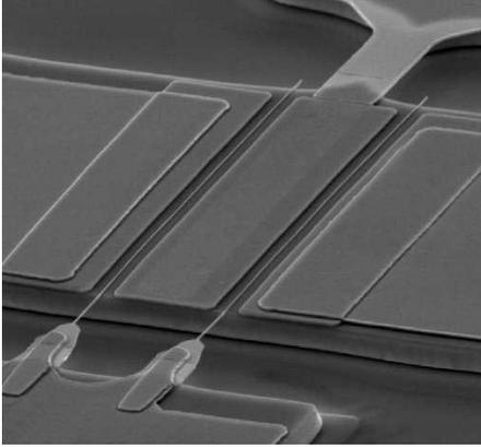
Figure 2. SEM micrograph of a two-finger InSb quantum well transistor with gate air-bridge at mesa edge.  $L_G = 0.1 \mu\text{m}$ ,  $L_{DS} = 1.0 \mu\text{m}$ .
