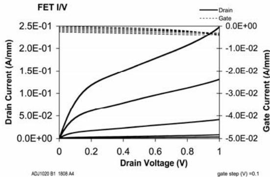
Figure 3.  $0.1 \mu\text{m}$   $L_G$  InSb QW transistor output characteristics at  $295 \text{ K}$ ,  $L_{DS} = 1 \mu\text{m}$ ,  $W_G = 40 \mu\text{m}$ ,  $V_{GS} = 0.1 \text{ V/step}$ .
