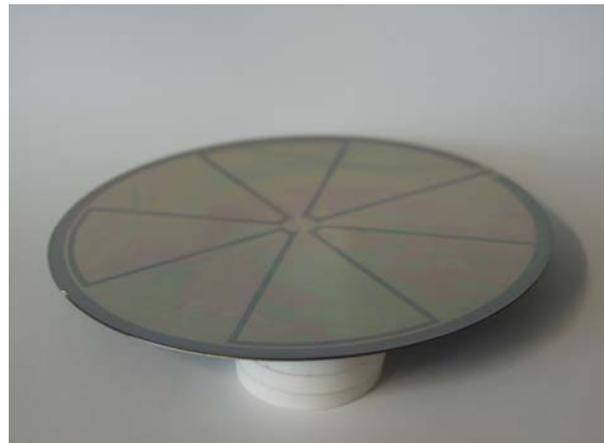
Fig. 3: Electrostatic carrier based on silicon wafer.
