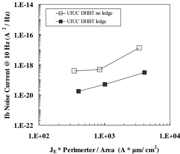
Figure 6: Comparison of effective base noise current at 10 Hz vs. Emitter current density times perimeter over area ratio
