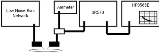
Figure 2: Low frequency noise setup. The ammeter can be switched out of the measurement path during actual measurement.
