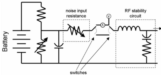
Figure 3. The RF stability circuit presents a 50 ohm impedance to the input of the device at RF frequencies. The left capacitor shorts the bias resistors so that noise input resistor can control what impedances are presented at noise measurement frequencies. The ammeter and voltmeter can be switched out of the measurement path during measurement.
