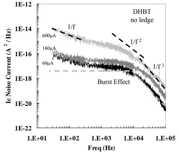
Figure 4: DHBT without ledge low frequency noise with  $I_E = 60, 160, 600\mu A$
