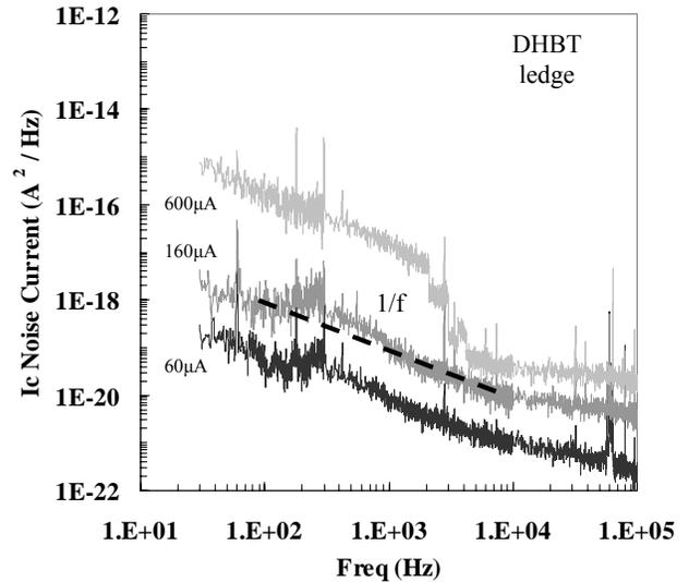
Figure 5: DHBT with ledge low frequency noise with  $I_E = 60, 160, 600\mu A$
