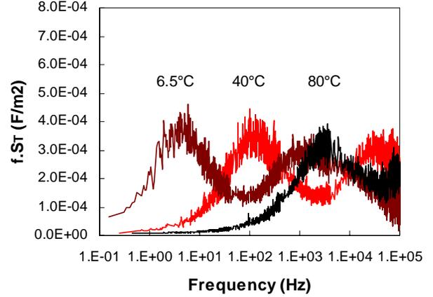
Figure 9. Evolution of the  $fS_V$  noise spectrum with temperature in a cross-shaped MIS device, highlighting the individual Lorentzian contributions.
