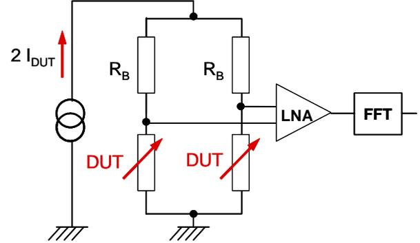
Figure 2. Differential measurement of the noise PSD of a 2-terminal device in a Wheatstone bridge configuration.
