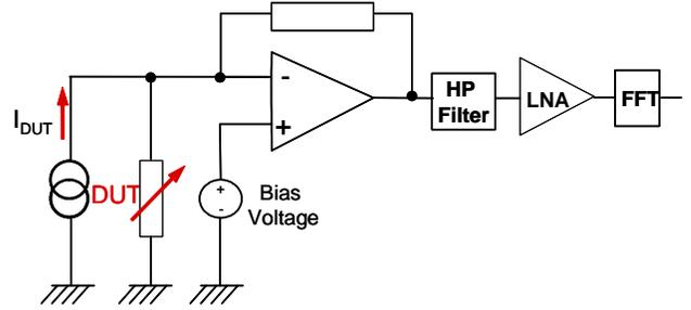
Figure 3. Single-ended measurement of the noise PSD of a 2-terminal device using a dedicated electronic circuitry.
