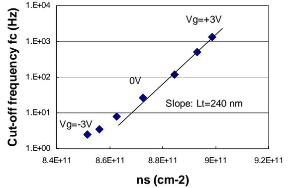
Figure 10. Drift of the cutoff frequency of the low-frequency peak in Fig. 9 as a function of the electron concentration in the channel. The slope provides the distance between the channel and the trap, according to Eq. (7).
