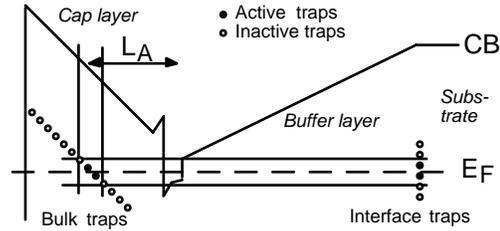
**Figure 1.** Band diagram of a P-HEMT-like planar device showing hypothetical bulk and interface traps. Only those in the vicinity of  $E_F$  are active.
