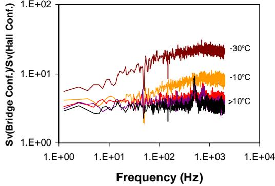
**Figure 5.** Ratio of the noise PSD of the same given device measured in the Wheatstone bridge and cross configuration. An additional noise contribution from the ohmic contact region perturbs the noise spectrum at low temperature in the former case, but not in the cross configuration.
