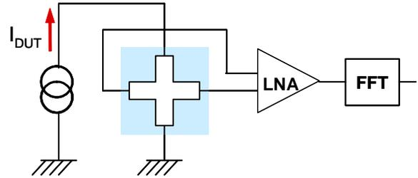
Figure 4. Differential measurement of the noise PSD using a cross-shaped device.
