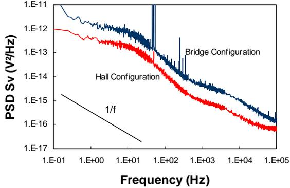
**Figure 6.** Comparison of the noise PSD of the same device measured either using 2 terminals in a Wheatstone bridge configuration or using all 4 terminals in the cross configuration.
