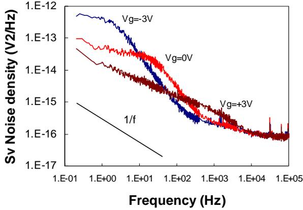
Figure 8. Evolution of the noise spectrum when varying the gate voltage in a cross-shaped MIS device. For the sake of clarity only 3 spectra were drawn.
