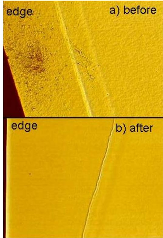
**Figure 5.** Optical microscope images of the wafer edge after pHEMT growth a) before platen modification and b) after platen modification. The edge particles are seen on the edge exclusion area of the wafer that has a width of 2.5 mm.
