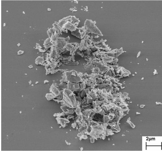
**Figure 1.** SEM image of crushed edge particle. The debris easily migrates into the device area.
