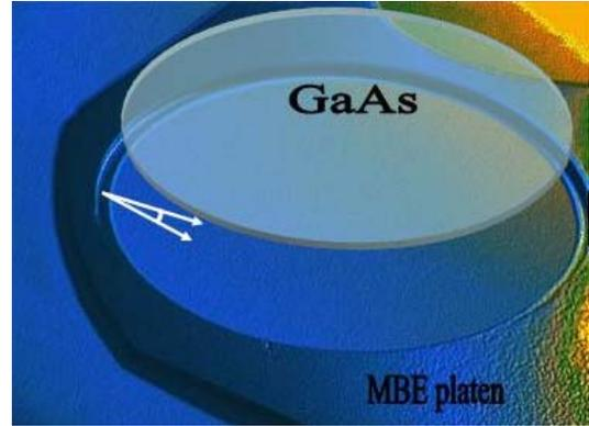
**Figure 4.** Modified MBE platen which has beveled edge in order to enable As beam access to edge of wafer. The white arrow indicates the beveled angle.
