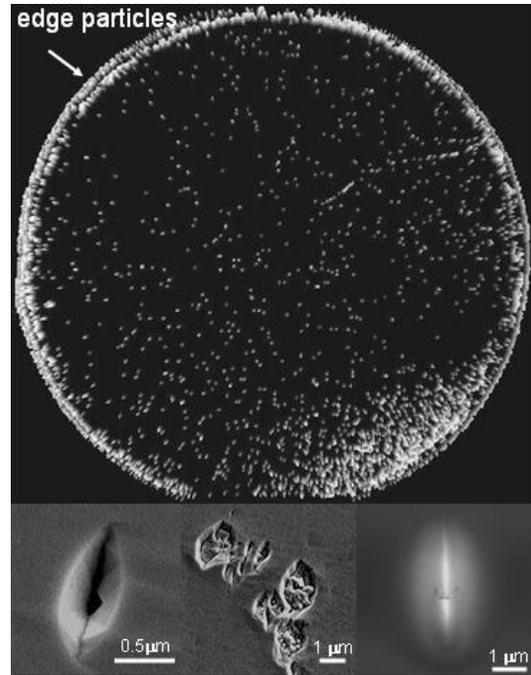
**Figure 2.** Particles on a 4-inch pHEMT scrapped wafer showing a high density of edge particles. The bottom insets show various oval defects in the active film side.
