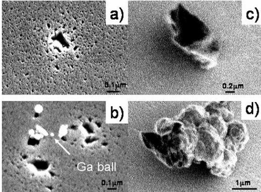
**Figure 3.** Various edge particles showing the formation of edge particles. Note that the Ga balls are formed near the pits and develop into edge particles.
