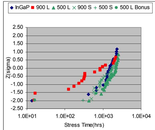
Fig. 6: Cumulative failures transformed into linear space for control and InGaP/InGaAsN variants.  $Z=0$  is equivalent to MTTF. The number in the legend indicates the base thickness and the letters S and L denote standard or low burn-in material.
