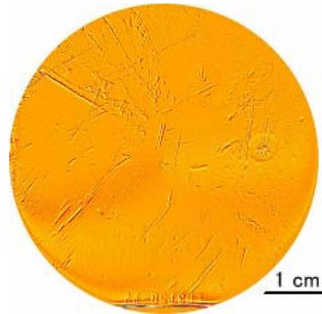
Figure 1 Surface morphology of epi HEMTs on 2 inch epitaxial wafer image
