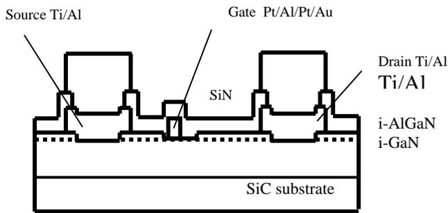
Figure 3 Schematic cross-section of HEMT device
