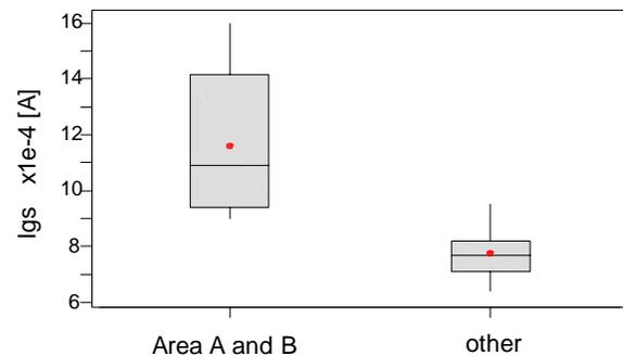
Figure 7 Box plot of gate leakage current comparing A, B area and other area
