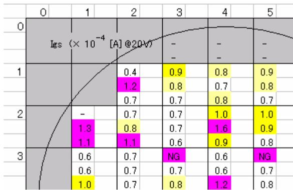
Figure 4 Map of gate leakage current on wafer
