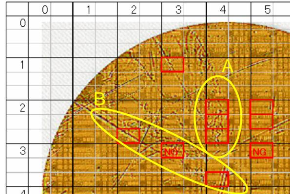
Figure 6 Defects concentrated area encircled A and B Gate leakage current devices are shown in square.
