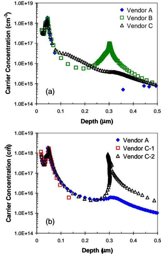
Figure 2. Polaron E-CV plots of two separate, (a) and (b), LM-HEMT growths in the  $3 \times 4$  in. configuration. The charge peak seen at the left, near the epiwafer surface, in all six samples is from the Si atomic planar doping and the InGaAs channel. The peak seen at a depth of  $0.3 \mu\text{m}$  in some of the samples is due to a charge accumulation at the epilayer-substrate interface.
