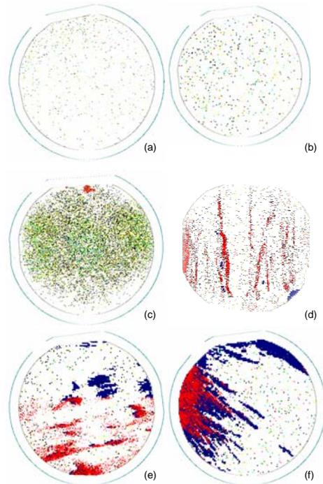
Figure 1. Surfscan 6220 defect maps for InP-HBT structures grown on substrates from (a) Vendor B, (b) Vendor C, (c) Vendor A, (d) Vendor D, (e) and (f) Vendor C. The maps compare uniform distributions typical of MBE (a, b) with unusual defect patterns related to substrate problems (c – f).
