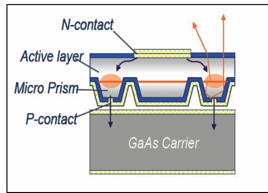
Fig. 3: Schematic view of a Thin Film LED
