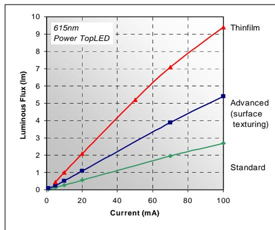
Figure 5: The influence of new technologies as surface texturing and Thin Film technology (615nm) with buried micro reflectors on the luminous Flux of a LED.
