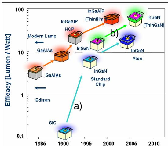
Fig. 2: Efficacy evolution of InGaAlP and InGaN LED-chips in the last decade, a) InGaN blue, b) InGaAlP green
