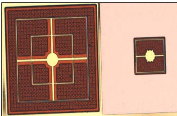
Figure 4: Top view on a 1mm thin film chip and a 300µm chip directly near by each other on the same wafer (buried micro reflector). This demonstrates the scalability of our Thin Film technology.
