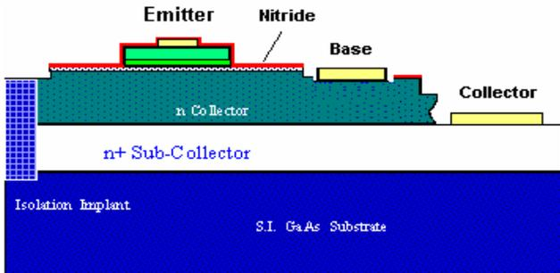
**Figure 2: HBT transistor showing thin nitride film and base contact.**
