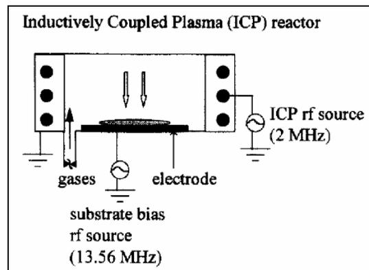
Figure 1: ICP etch system showing both RIE and ICP power source.
