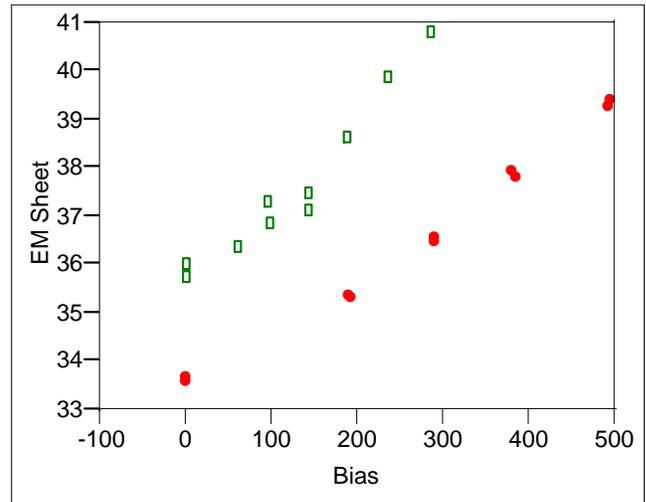
**Figure 4: Bias voltage of the plasma plotted against emitter sheet resistance.**
