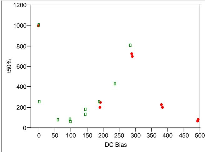
**Figure 5: Bias voltage versus  $t_{50\%}$  including control wafers that were not exposed to plasma damage. The data overlap between the two lots processed two months apart confirms the cusp in the data.**
