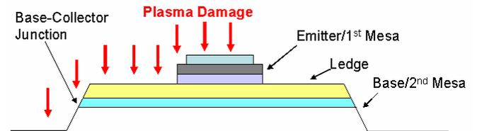
**Figure 6: Plasma exposure pattern to emitter and base.**
