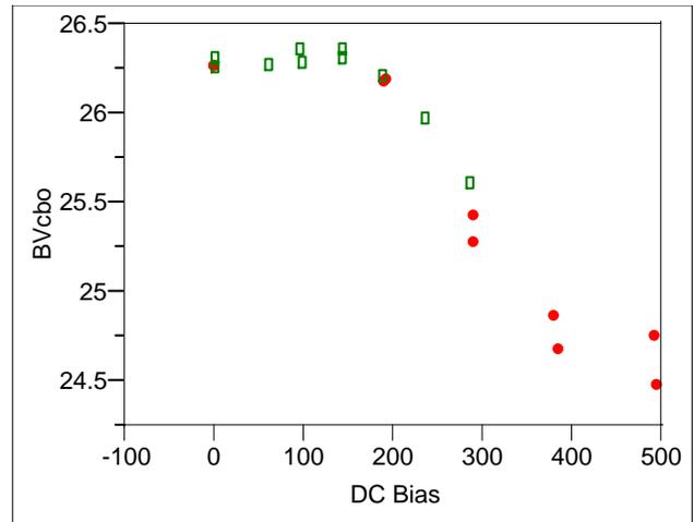
**Figure 3: DC Bias plotted against the collector-base breakdown voltage.**
