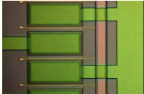
Figure III.CSN-1 4000A for protection layer, after HAST test
