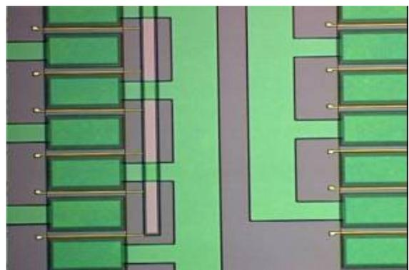
Figure IV.CSN-2 4000A for protection layer, after HAST test
