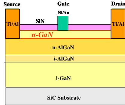
Fig. 1 Schematic drawing of the surface-charge-controlled n-GaN-cap structures. Thin n-type GaN cap layer was grown on AlGaIn/GaN structure. SiN passivation was formed on GaN cap layer between electrodes.
