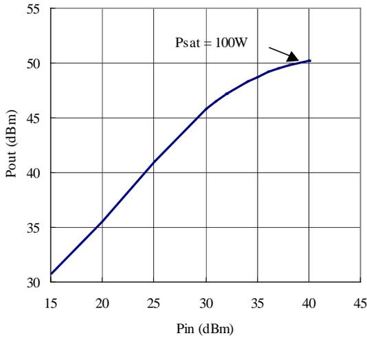
Fig. 5 Pulsed CW power measurement results of single-chip AlGaIn/GaN HEMT amplifier at 2.14 GHz. Quiescent drain current is 500 mA at  $V_{ds} = 50$  V.
