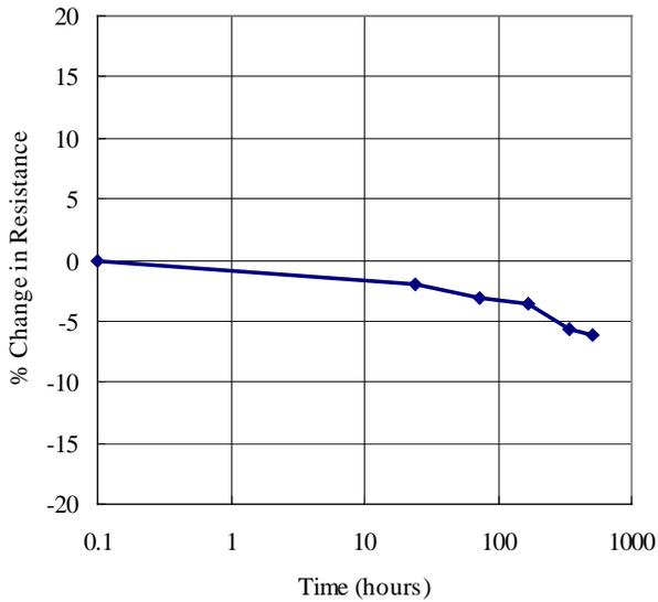
Fig.9 Resistance variation of ohmic electrodes under current density of  $2 \times 10^6$  A/cm<sup>2</sup> at 250 deg-C in nitrogen ambient.
