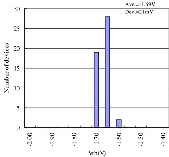
Fig.7 Histogram of threshold voltage for fabricated AlGaIn/GaN HEMT
