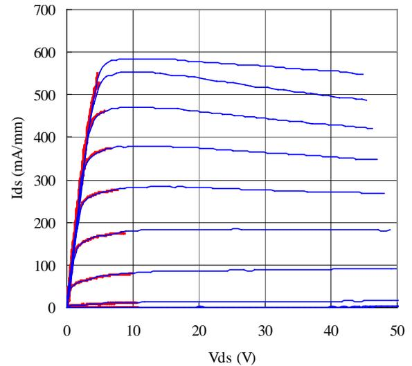
Fig. 3 Comparison of I-V characteristics at 10 V and 50 V operations using a 100-Hz curve tracer. The gate width was 40  $\mu\text{m}$ . The gate voltage was swept from +2 V to -2.5 V with 0.5 V step.
