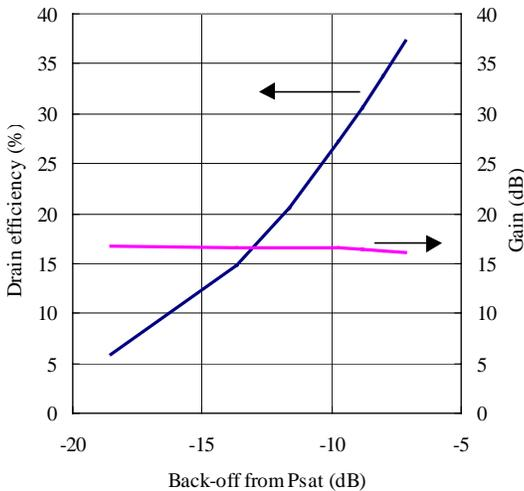
Fig.6 Single-tone W-CDMA RF performance of AlGaIn/GaN HEMT measured at 2.14 GHz. Bias condition is  $V_{ds} = 50$  V,  $I_{dsq} = 500$  mA.
