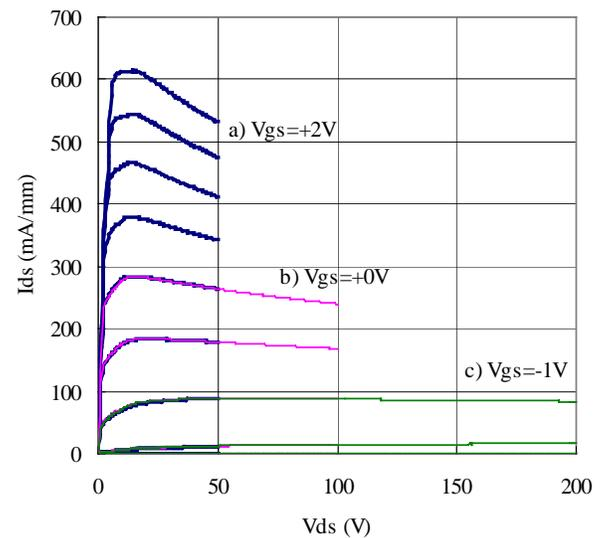
Fig. 4 I-V characteristics of 40- $\mu\text{m}$  gate periphery using a semiconductor parameter analyzer. The gate voltage was swept a) from +2 V to -3 V with 0.5 V step up to  $V_{\text{ds}}$  of 50 V, b) from +0 V to -3 V with 0.5 V step up to  $V_{\text{ds}}$  of 100 V, c) from -1 V to -3 V with 0.5 V step up to  $V_{\text{ds}}$  of 200 V.
