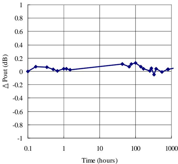
Fig.10 Power characteristics under P<sub>3</sub> dB RF-stress test at 60 V.
