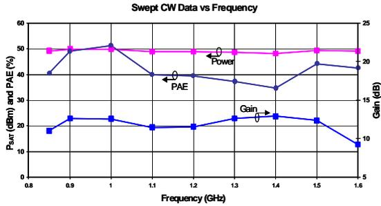
Figure 3: Measured broadband power performance of a Cree CRF-24060 commercial 60 watt transistor
