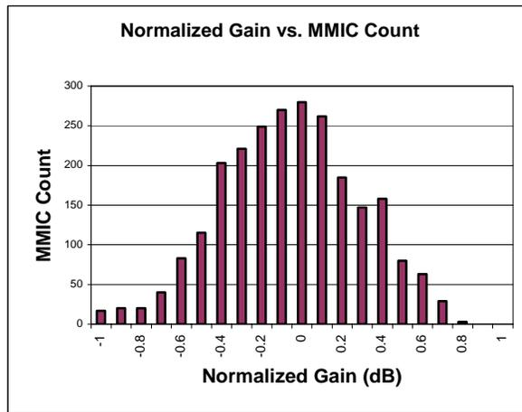
Figure 7: Distribution of small signal gain for over 2,400 high power SiC MMICs produced across six 3-inch wafers lots
