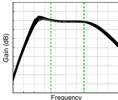
Figure 6: Small signal gain overlay for 70 high power MMICs on a single SiC wafer.
