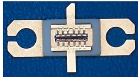
Figure 2: Cree CRF-24060 commercial 60 watt transistor shown without the lid.
