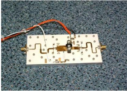
Figure 4: CRF-24060 60 watt transistor evaluation circuit
