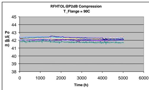
Figure 5: RF Operating Life data on fifteen 10 Watt SiC MESFETs operating at  $T_j = 140^\circ\text{C}$  showing no degradation after 5,000 hours.
