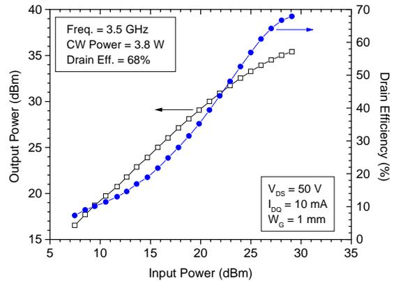
Figure 1: On-wafer CW load pull measurement of SiC MESFET with 3.8 W/mm and 68% drain efficiency.
