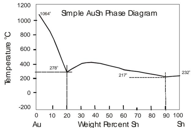
Fig.1- Au-Sn phase diagram
