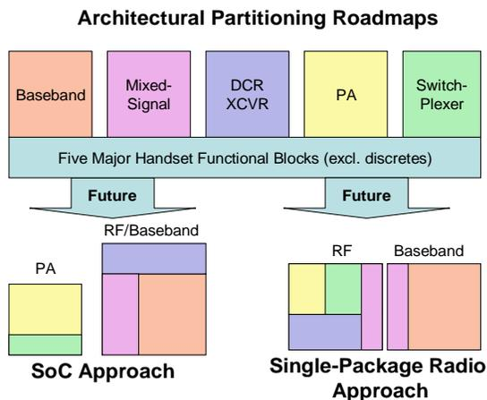
Fig. 1: SoC approach compared to SPR approach
