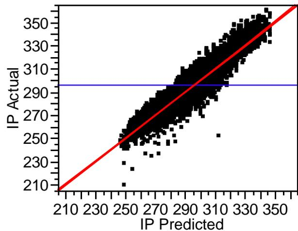
Figure 8. Example of multivariate least-square fit showing that the MVM prediction matches measured values of  $I_{peak}$  with an  $R^2$  fit of 0.88. The MVM prediction for BV matches measured values with an  $R^2$  fit of 0.92.
