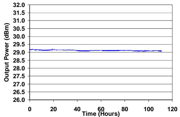
Figure 5 Output power stability of a 4mm FET with 10:1 load mismatch at drain bias of 30V. Power changed less than 0.1 dB over the duration of the test.
