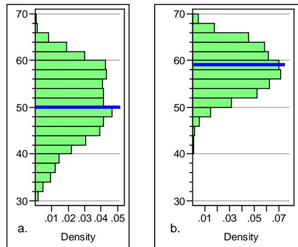
Figure 4. HVMFET breakdown voltage (vertical scale) distribution from production wafers tested (a) before and (b) after the GCFP is applied. The FP produces a typical increase in BV of about 15% and also reduces BV variability wafer-to-wafer by 60%.
