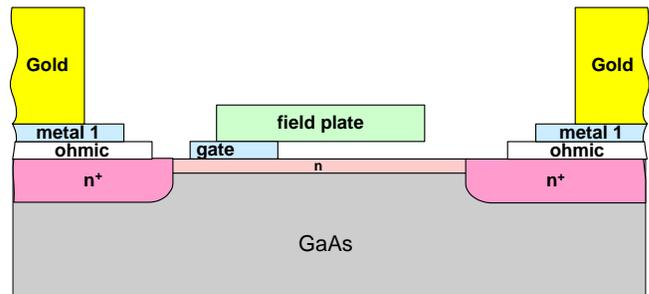
Figure 1. Cross section drawing of HVMFET showing Gate-Connected Field Plate (GCFP). Region under the field plate is filled with passivation dielectric.
