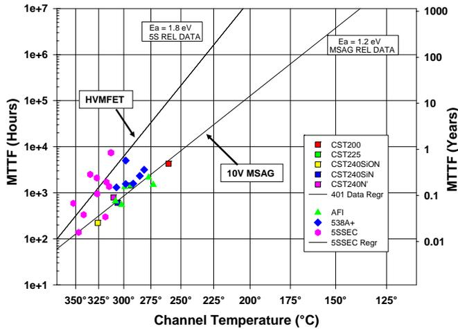
Figure 6. Arrhenius plot for the temperature-accelerated life test data shows extrapolated MTTF of  $> 10^7$  hours at 150°C for the HVMFET.
