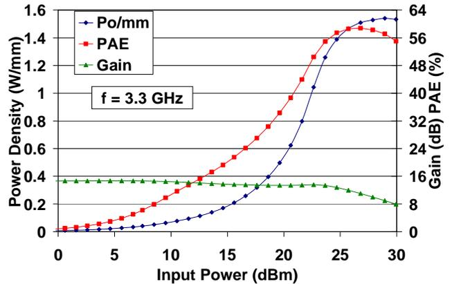
Figure 3. Typical load-pull results measured at 3.3 GHz for a 4mm HVMFET at 28V drain bias. Tuned for power, maximum output power density is typically 1.5W/mm with PAE up to 60%.
