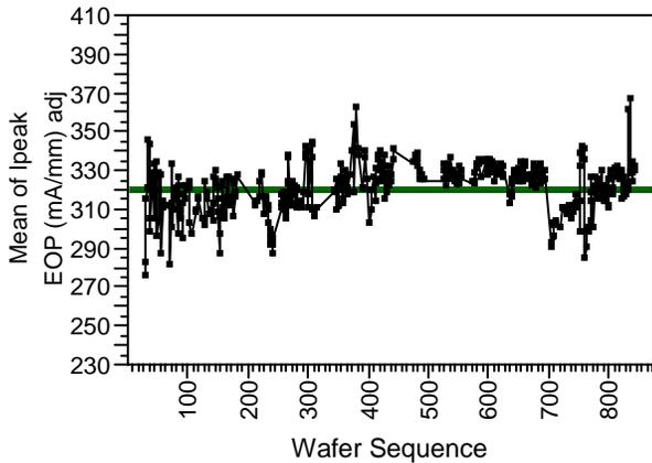
Figure 9. Run chart of Ipeak for standard-process HVMFET wafers. The median wafer-average value of Ipeak is 321 mA/mm and the standard variation wafer-wafer is less than 4%.
