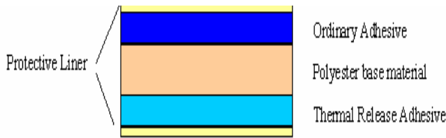
Figure 2. Construction of Thermal Release Adhesive Tape
