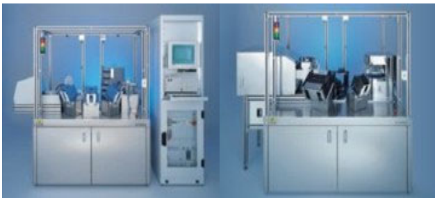
Figure 8. EVG850 bond and de-bond systems (with kind permission).
