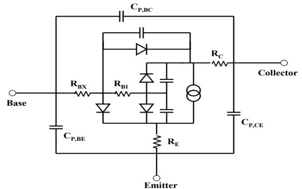
Figure 1. Topology of the DHBT large-signal model
