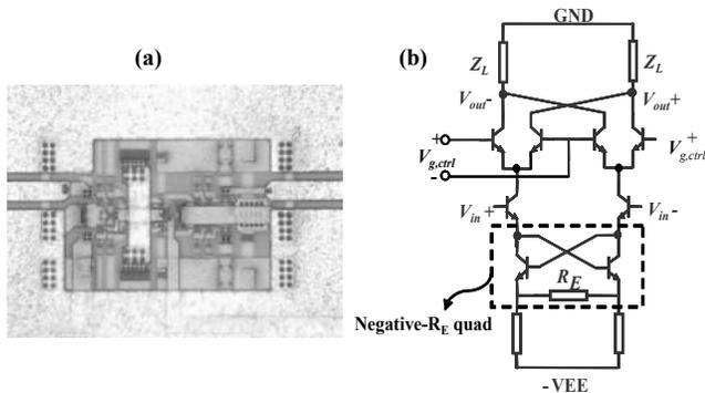
Figure 6. (a) Photograph of the core high-gain, wideband VGA (b) schematic of the modified Gilbert cell using negative resistance
