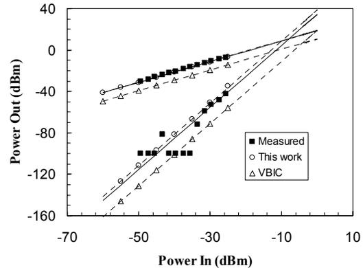
Figure 8. Two-tone measurement data at 30GHz with 19dB VGA gain. VBIC and SDD model simulation results are compared.
