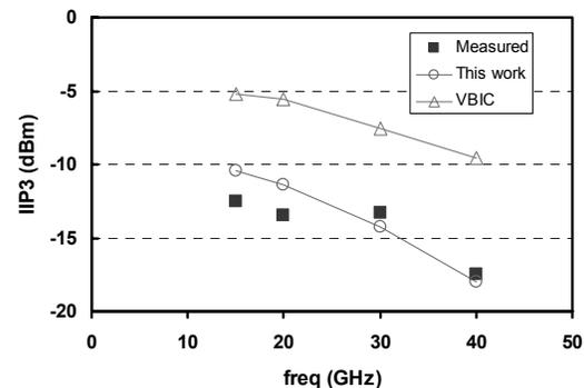
Figure 9. Model comparison of the two-tone nonlinearity results when the VGA gain is 21dB.
