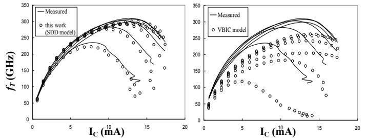
Figure 5. Measured and modeled  $f_T$  as a function of collector current for  $0.5 \times 4.0 \mu\text{m}^2$  VIP2 InP/InGaAs DHBT. The model developed in this work (left) shows better  $f_T$  trend fittings than VBIC model (right) does.
