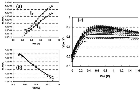
Figure 2. Modeling results of large-signal model developed in this work for  $0.5 \times 4.0 \mu\text{m}^2$  VIP2 InP/InGaAs DHBT. The solid lines represent measured data and the circle marks represent the model data. (a) Gummel plot, (b) reverse Gummel plot, and (c)  $V_{BE}$  curves vs.  $V_{CE}$ .
