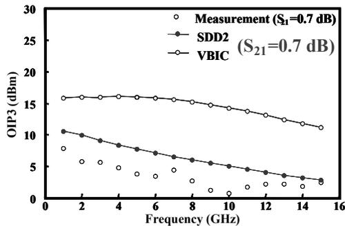
Figure 7. One-tone measured and modeled results when the gain is 0.7dB.
