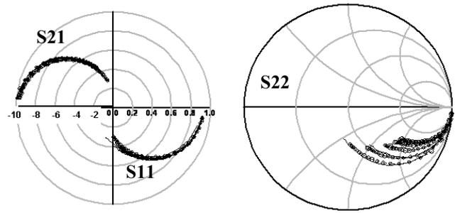
Figure 4. Measured and modeled S-parameters of  $0.5 \times 4.0 \mu\text{m}^2$  InP DHBT at  $V_{CE} = 0.6$ - $1.6$  V,  $J_C = 2.1 \text{ mA}/\mu\text{m}^2$ . The solid lines represent measured data and the circle marks represent the model data.
