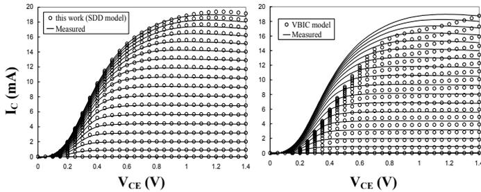
Figure 3. The measurement data of  $0.5 \times 4.0 \mu\text{m}^2$  VIP2 InP/InGaAs DHBT compared with the simulations of model developed in this work (left) and the VBIC model (right).
