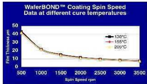
Figure 1. WaferBOND™ adhesive spin-speed curve showing single-coating thicknesses ranging from 10-40 μm. The viscosity is 1050 cP. Coating is on 100-mm silicon using 3 ml of WaferBOND™ adhesive. The spin was for 30 seconds at 5000 rpm acceleration. Films were baked for 120 seconds at 100°C followed by noted temperature for 120 seconds, and measured on an AlphaStep 200 profilometer.
