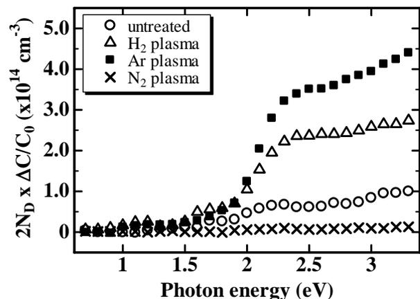
Fig. 3. photocapacitance spectra taken from the Ni/*n*-GaN Schottky diodes with and without plasma treatment for 60 min.
