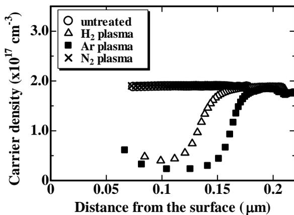
Fig. 2. Depth profiles of the carrier density for the Ni/*n*-GaN Schottky diodes with and without plasma treatment.
