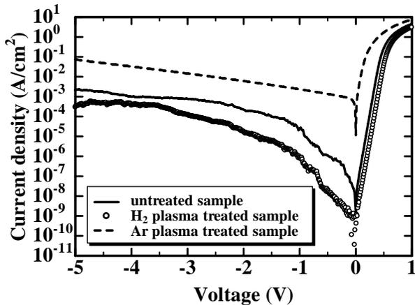
Fig.1. *I-V* characteristics of Ni/*n*-GaN Schottky diodes with and without plasma treatment.
