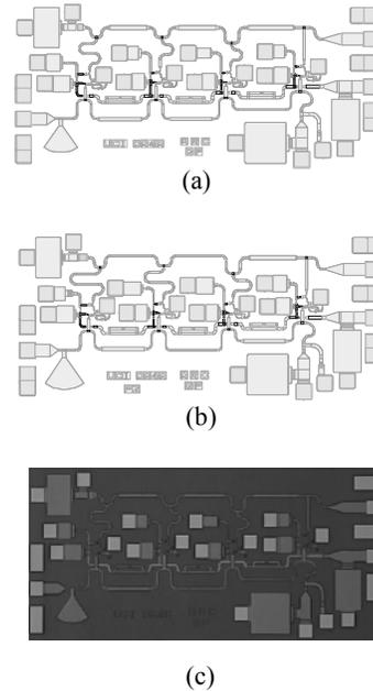
Figure 6: (a) The layout of 4-stages DA in lower  $f_{max}$  and higher  $\beta_0$  and  $f_t$  process, (b) The layout of 4-stages DA in slightly higher  $f_{max}$  and lower  $\beta_0$  and  $f_t$  process, and (c) The chip microphotograph of DA in Fig. 6(a).
