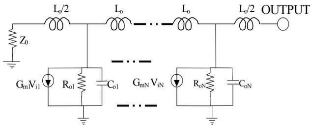
Figure 4: The artificial output transmission line of N-stage HBT DA with generic gain cells.
