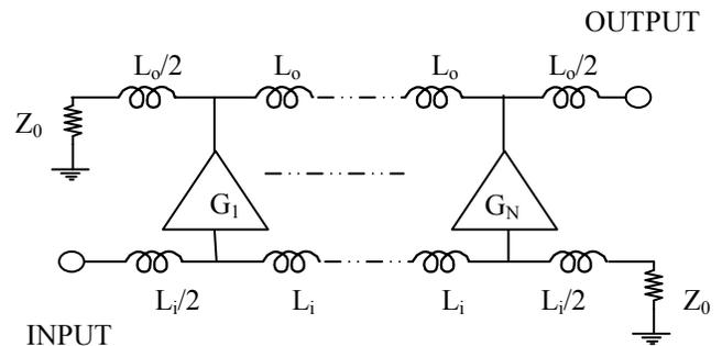
Figure 1: The schematic of N-stage HBT DA with generic gain cells.
