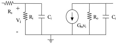
Figure 2: The equivalent small signal model of generic HBT gain cell.
