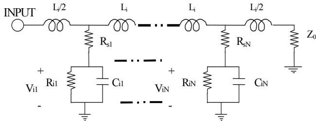
Figure 3: The artificial input transmission line of N-stage HBT DA with generic gain cells.
