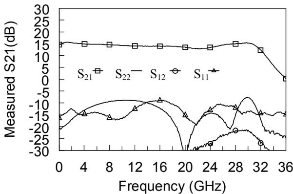
Figure 8: The measure S-parameters of DAs in Fig. 6(c).
