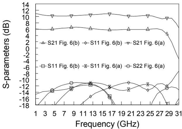
Figure 7: The S-parameters comparisons of DAs in Fig. 6(a) and 6(b).
