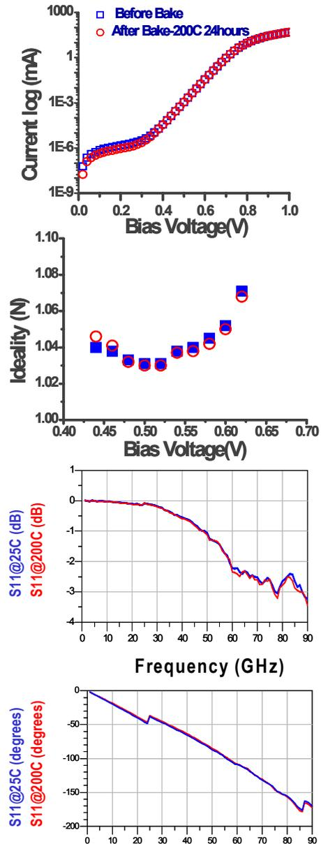
Figure 3 – Dc and S-parameter measurements (Magnitude and phase) comparison for before and after the 200C-24 hour bake cycle showing no degradation in the diode performance
