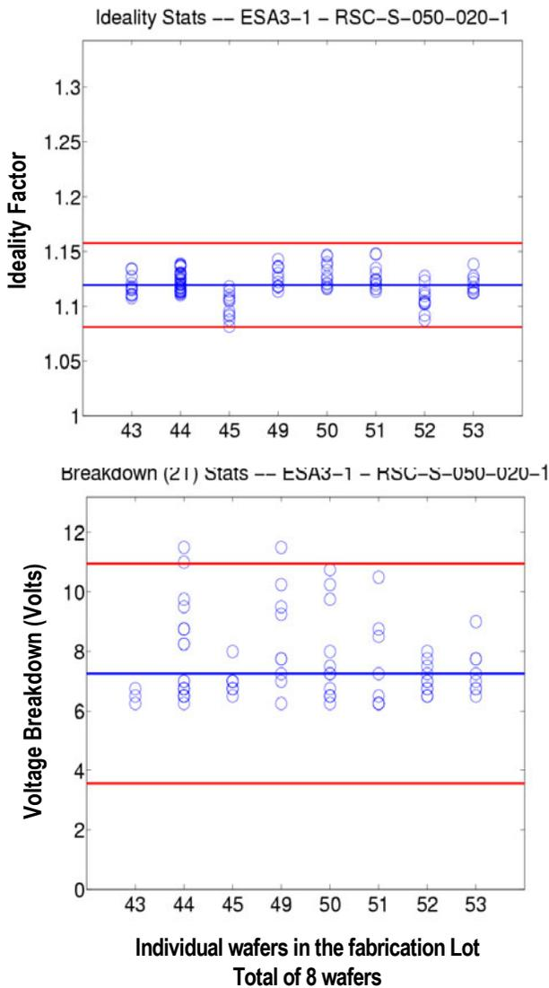
Figure 2- shows the statistical 5um(anode diameter) diode parameter map as a function of 8 processed wafers in the fabrication wafer lot. The data points are multiple measurements on various sites on each wafer. (Bottom) shows the voltage breakdown measured at 5μA reverse bias voltage. The lower limit is most important for device performance and set as 4 Volts for this particular diode design.
