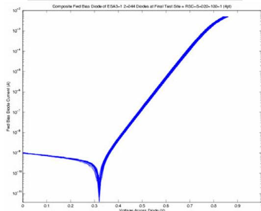
Figure 1 – Top- microscope photograph of the PAS diode with device sections marked. Bottom- Current voltage characteristics of 2UM anode PAS diodes plotted on top of each other from 40 sites across 4" GaAs wafer, showing very uniform characteristics
