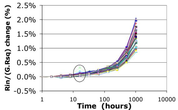
**Fig. 7 Temporal behavior (a) of the normalized quantity  $R_{in}/G \cdot R_{sq}$  at room temperature of a set of devices on a wafer aged at 275°C. Circled: temperature fluctuation “spike” cancellation due to normalization.**
