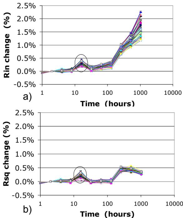
**Fig. 6 Temporal behavior (a) of the input resistance  $R_{in}$  at room temperature of a set of devices on a wafer aged at 275°C, (b) of their resistivity  $R_{sq}$ . Circled: “spike” due to the fluctuation of the measurement temperature.**
