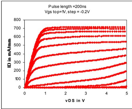
Fig.3: Pulsed I-V of 6" 0.1 $\mu$ m PHEMT
