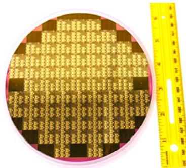
Fig.1: Fully processed 2-mil 6" 0.1 $\mu\text{m}$  PHEMT MMIC wafer.
