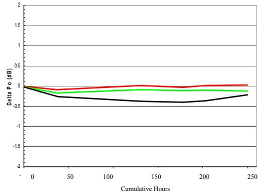
Fig.6.: Measured saturated power change during high temperature RF testing. T<sub>baseplate</sub> = 125°C, Tch=175C, Compression=4.5dB
