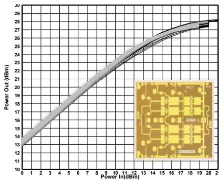
Fig.4: Measured Pout for 6" 0.1 $\mu$ m Power PHEMT MMIC (gray) compared with its typical 3" counterpart (black). Inset: Balanced V-Band MMIC using 0.1 $\mu$ m 6" power PHEMT technology. (Output stage = 8x200 $\mu$ m)
