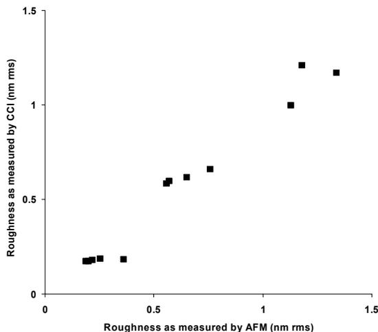
Figure 5 – CCI determined roughness values vs. AFM determined values
