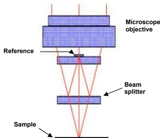
Figure 2 Schematic diagram of a Mirau type interferometer
