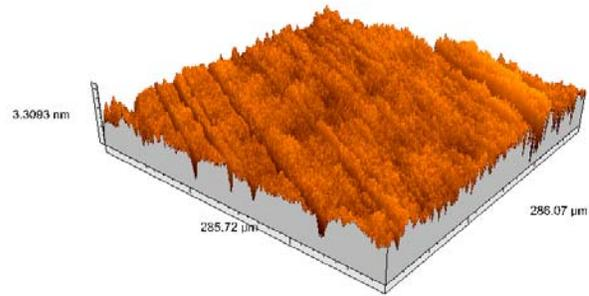
Figures 3a (top) & 3b– Pseudo-colour CCI images of ‘good’ (rms roughness 0.18 nm, average roughness 0.14 nm) and ‘damaged’ (rms roughness 0.35 nm, average roughness 0.28 nm) semiconductor substrates
