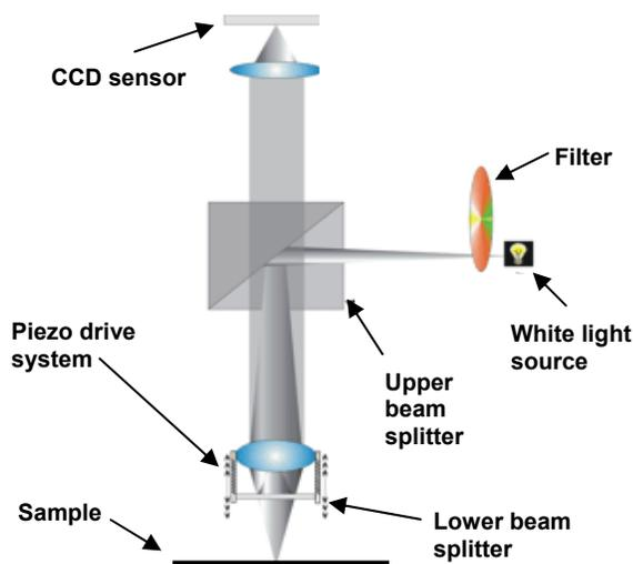
Figure 1 Schematic diagram of an interference microscope
