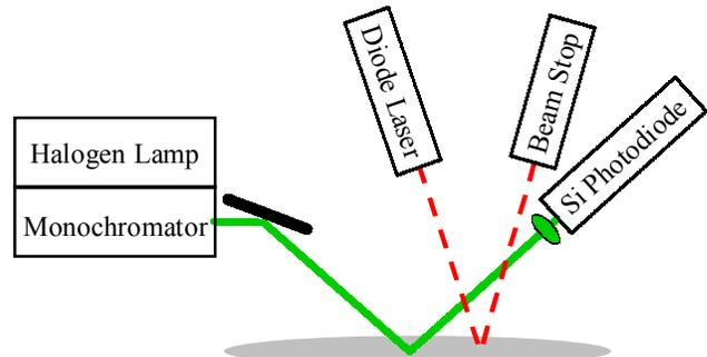
Figure 2. New optical layout for photoreflectance measurement.
