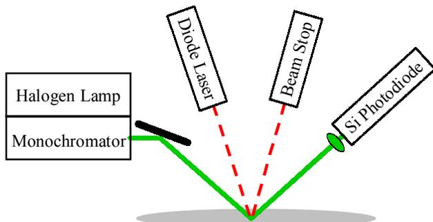
Figure 1. Typical optical layout for a photoreflectance measurement.
