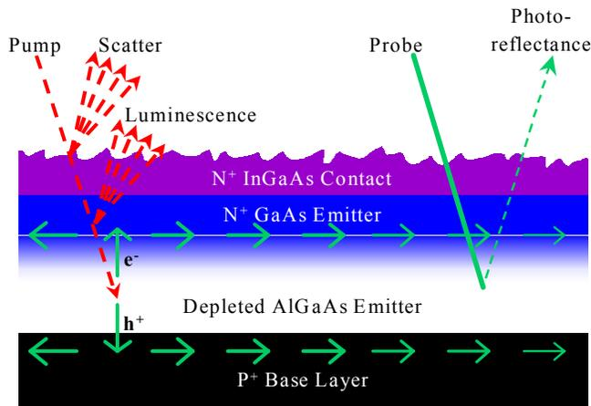
Figure 6. Schematic of carrier generation and lateral diffusion between the pump and probe beams.
