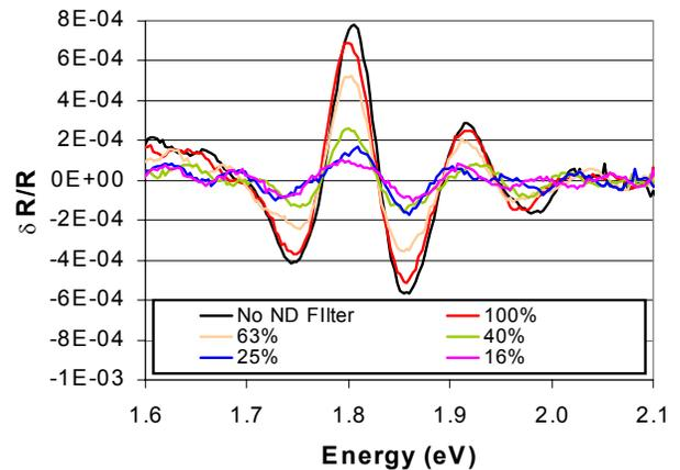
Figure 7. Overlay of the PR signal as a neutral density filter is used to reduce the intensity of the probe laser. The transmittance of the neutral density filter is listed in the legend.
