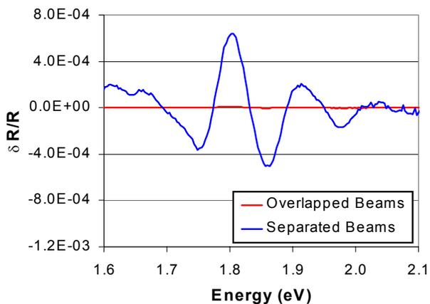
Figure 3. PR signal of product HBT wafer. Overlapped beams shows minimal noisy signal, while separating the beams 5 mm recovers a strong clear PR signal.
