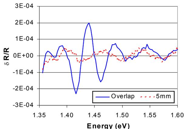
Figure 5. PR signal of undoped GaAs film on n+ GaAs showing strong signal when the beams are overlapped. No PR signal is observed after separating the beams by 5 mm
