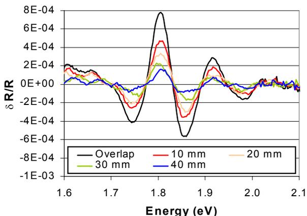
Figure 4. Overlay of the PR signal where the probe beam is in the center of the 100 mm wafer and the pump is moved toward the wafer edge.
