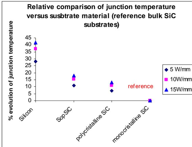
Figure 2 : maximal computed junction temperature as a function of the substrate nature. The comparison is drawn for a range of power density to be dissipated from 5 to 15W/mm.
