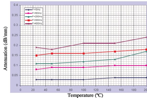
Figure 3: Characterization of RF losses in the poly-SiC substrates vs. temperature and frequency
