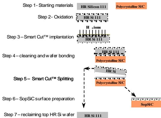
Figure 1: process flow applied to SopSiC substrate realization
