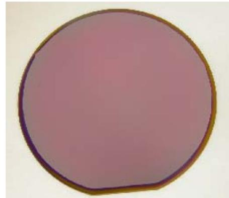
Picture 1: typical 100 mm SopSiC substrate obtained by the Smart Cut™ technology. As observed in this picture, an excellent layer transfer quality is obtained showing no large macroscopic bonding defects.
