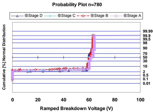
Figure 5 MIMCAP-On\_Via Breakdown Probability Plots At 4 Test Stages. Test Vehicle is a capacitor with area 1,057,000um<sup>2</sup>
