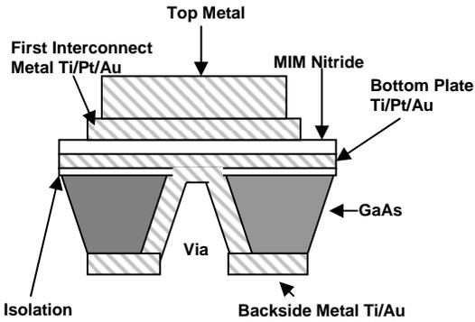
Figure 1 Cross Section of A Fully Processed MIMCAP Built On Top of Backside Via
