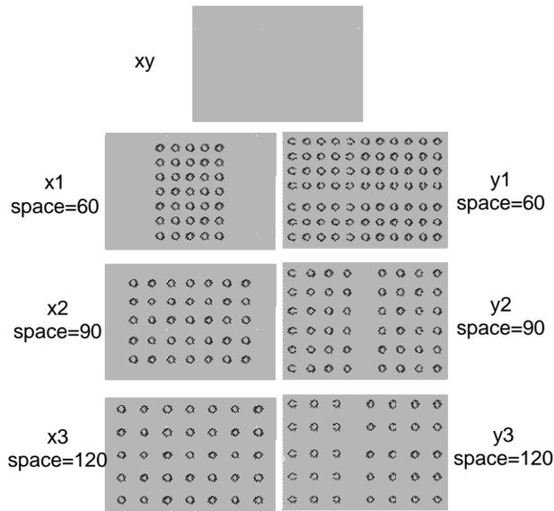
Figure 2 Backside Via Layout Pattern To Test Its Effect On Capacitor Performance
