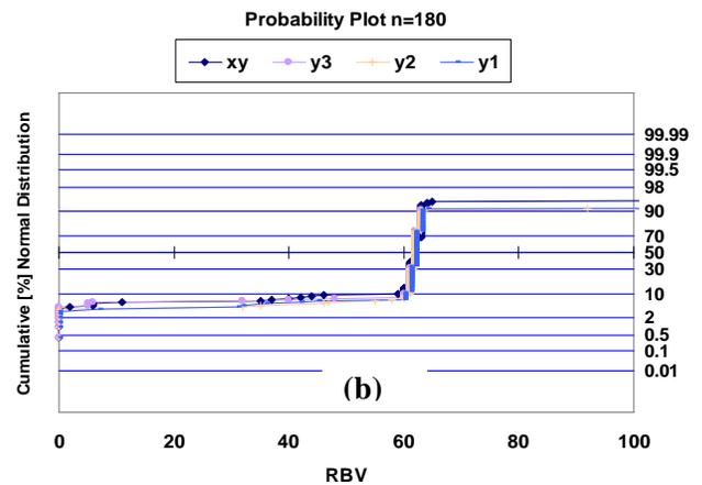
Figure 4 Capacitor Electrical Breakdown Probability Plots With Various Via Layout After Backside Process. Test Vehicle is a capacitor with area 1,057,000um<sup>2</sup>
