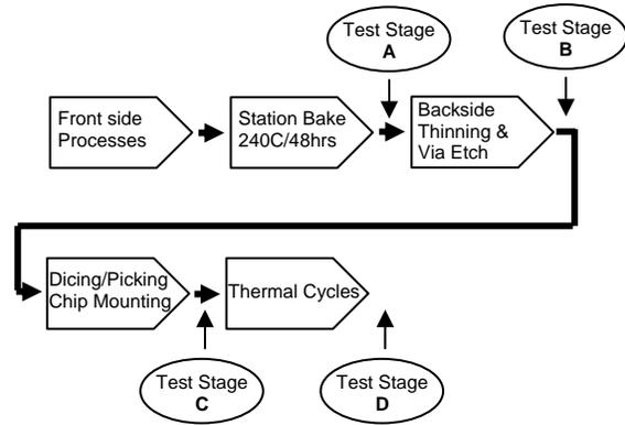
Figure 3 Fabrication Process Flow And Test Stage Setup
