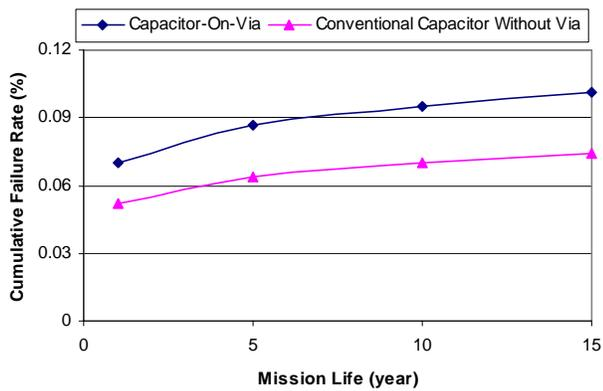
Figure 6 Reliability Prediction For Both MIMCAP-On-Via And Conventional MIMCAP Without Via After Thermal Cycles
