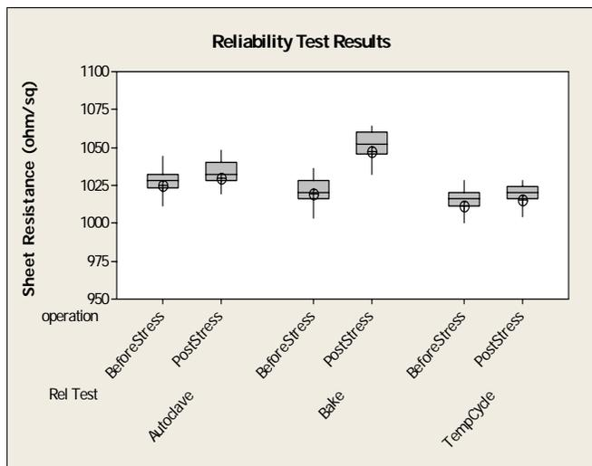
**Figure 2. Reliability test results for the optimized WSi film. Each group contains approximate 150 test points. The bake test produces a 2.5% shift in sheet resistance.**
