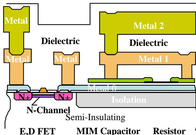
**Figure 3. Process integration method for the high value resistor.**
