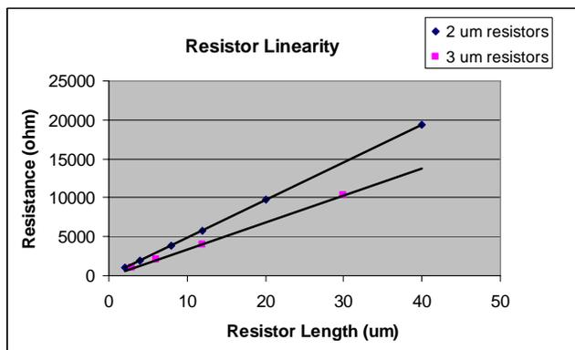
**Figure 4. Resistor series with 2 and 3 μm width plotted against the layout length of the elements.**
