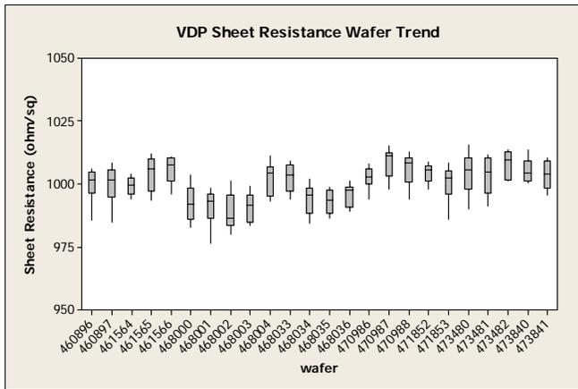
**Figure 5. Pilot line sheet resistance measurement trend demonstrates capable process.**
