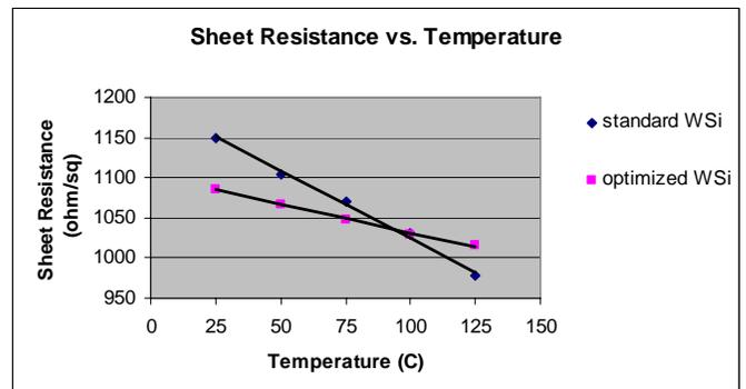
**Figure 1. TCR measurements for WSi thin film resistors. Standard WSi film exhibits a -1500 ppm/ $^{\circ}\text{C}$  TCR while the TCR of the optimized film was measured at -650 ppm/ $^{\circ}\text{C}$ .**
