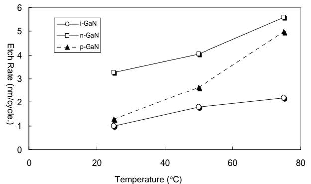
Figure 3. GaN K<sub>2</sub>S<sub>2</sub>O<sub>8</sub>/KOH binary etch rate vs. temperature.
