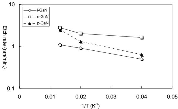
Figure 4. GaN K<sub>2</sub>S<sub>2</sub>O<sub>8</sub>/KOH binary etch rate Arrhenius law.
