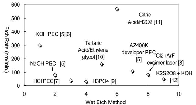
Figure 1. Etch rate of several etching techniques.
