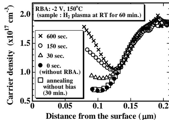
Fig. 3. Time variation of the carrier depth profiles for the H<sub>2</sub> plasma treated Ni/n-GaN Schottky diodes with RBA at 2 V.
