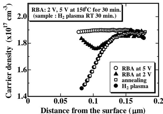
Fig.2. Depth profiles of the carrier concentration for the H<sub>2</sub> plasma treated Ni/n-GaN Schottky diodes after the RBA at 2 and 5 V.
