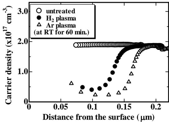
Fig. 1. Depth profiles of the carrier density for Si-doped GaN with and without plasma treatment.
