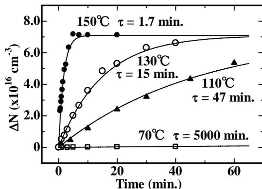
Fig. 4. Time variation of the recovered carrier concentration at the 100 nm depth from the surface for the H<sub>2</sub> plasma treated Ni/n-GaN Schottky diodes with RBA at 2 V at the different temperatures.
