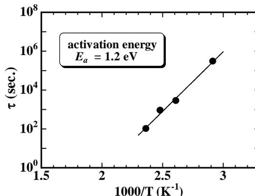
Fig. 5. Arrhenius analysis of the 2-V-RBA dissociation time for the Si-defects complexes in the H<sub>2</sub> plasma treated Ni/n-GaN Schottky diodes
