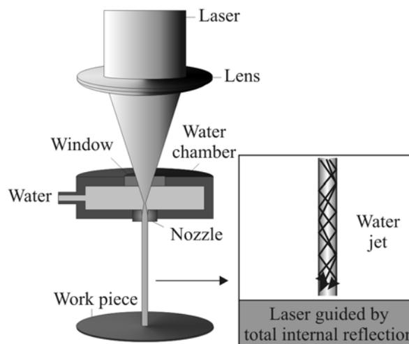
**Figure 1** Water-jet-guided laser
