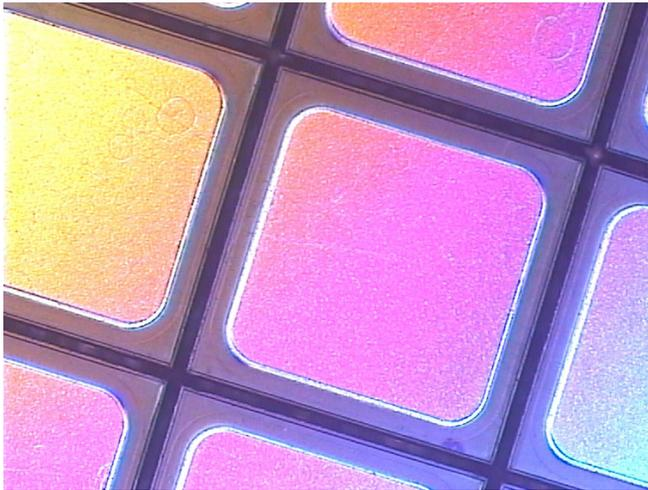
**Figure 2** Through-cutting of a thick SiC wafer
