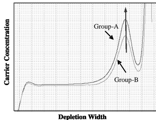
Figure 3: C-V profiles of Emitter-Base of BiFET wafers. Group-A and Group-B wafers come from different MOCVD growth runs.
