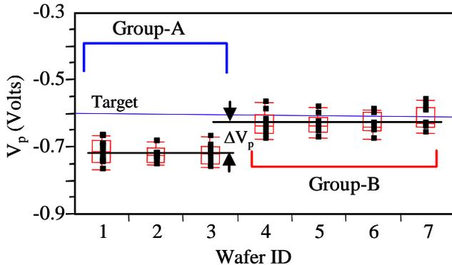
Figure 4: Pinch off voltage  $V_p$  vs Wafer ID of a depletion mode FET from a single fabrication run. Note the  $\Delta V_p$  of 100 mV between two groups arise due to difference in epitaxial layers resulting.
