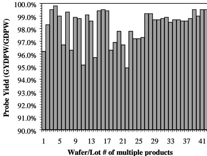
Figure 7: DC probe yield as a function of wafer/lot numbers collected over time. Gross Yielding Dies per Wafer is computed after performing a series of DC tests for both HBT and FET active devices as well as passives such as resistors, and capacitors in the design.
