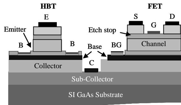
Figure 1: Schematic cross section of an integrated HBT and FET. S, D, G, BG are the source, drain, gate and back-gate contacts of the FET and E, B, C are emitter, base, and collector contacts of the HBT respectively.
