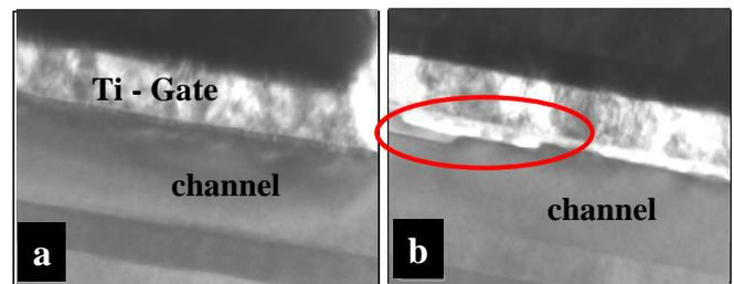
Figure 6: Transmission Electron Micrographs of the Gate region. Image (a) is from the gate Schottky with  $n=1.23$  and image (b) is from the non-ideal Schottky contact with  $n>2$ . Note the sinking gate, highlighted in image (b).
