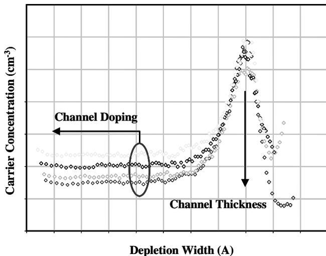
Figure 2: C-V profile of Emitter-Base in a BiFET wafer. Different curves are collected from a set of DOE wafers with different doping concentrations.
