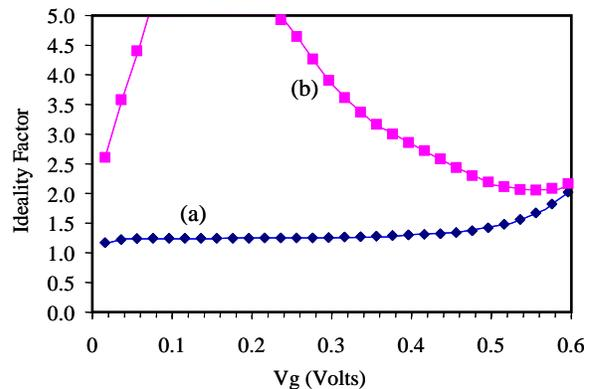
Figure 5: Ideality factor as a function of gate voltage of the Schottky contact. Curve (a) is generated from a FET with good electrical characteristics and curve (b) is generated from a FET with poor electrical characteristics.
