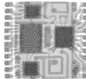
**Figure 2 – TriQuint Semiconductor 6mm x 6mm Transmit Module X-ray (TQMxx4002)**
