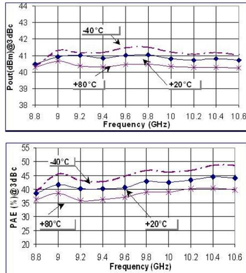
Figure 9. 11W output power X-Band MMIC for phased array applications. Output power and PAE for three ambient temperatures (-40, +20, +80degC) measured in a test jig.
