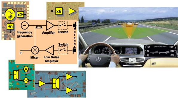
Figure 8. Typical line up of an ACC long-range radar at 77GHz based on UMS MMICs.
