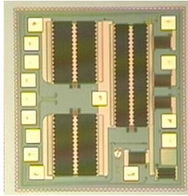
Figure 3. FMS2028, quad-band GSM - SP6T switch, 852 x 990  $\mu\text{m}$
