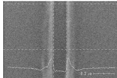
Figure 5. SEM image of the gate dimensions in resist before and after it has been shrunk to 128nm
