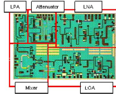
Figure 4. Highly integrated receiver operating between 17-23 GHz
