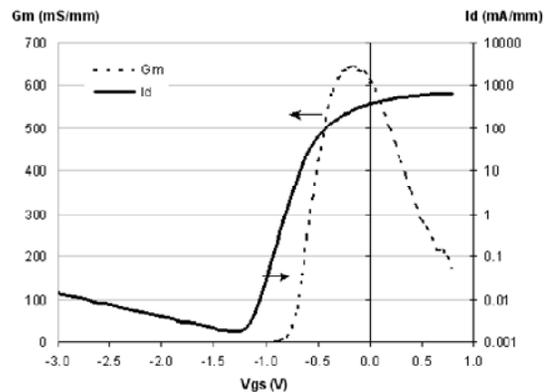
Figure 5. On wafer PHEMT transfer curve
