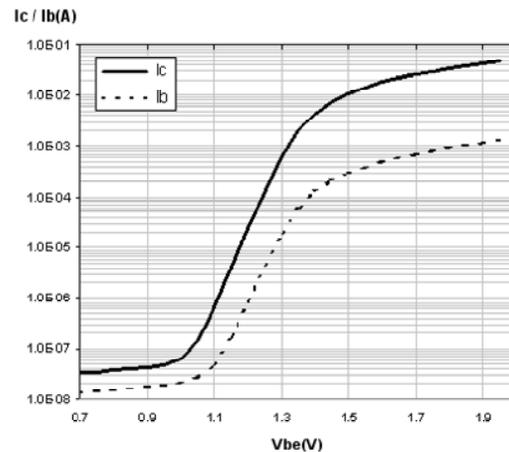
Figure 6. On wafer HBT Gummel plot
