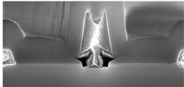
Figure 1. Cross-section of a PH25 device
