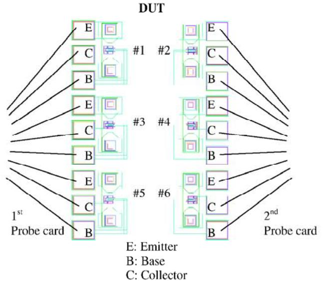
Figure 4. Schematic view of HBT pattern: 6 transistors with probe card connections.
