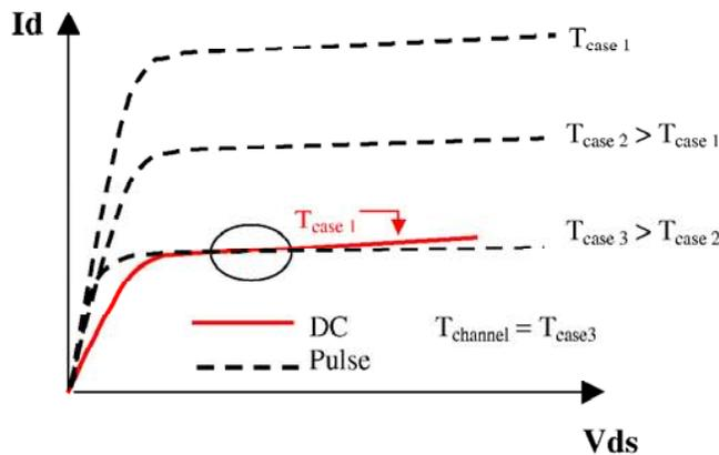
Figure 7. Pulse measurement method
