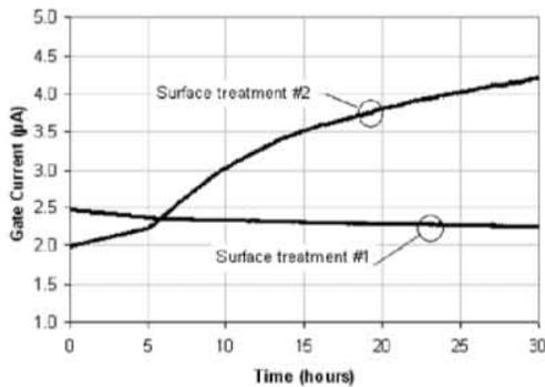
Figure 9. Evolution of the gate current on PHEMT transistor with different surface treatments
