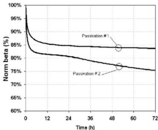
Figure 10. Evolution of the normalized beta of a HBT transistor with two different types of passivation
