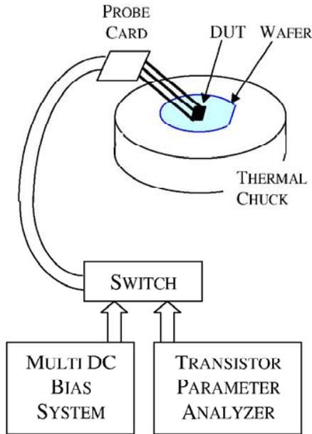
Figure 3. WLR system general schematic
