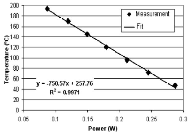
Figure 8. Rth of the HBT transistor
