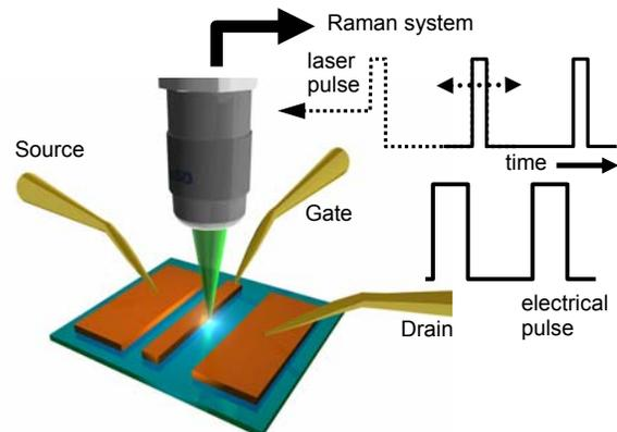
FIGURE 1: Schematic of nanosecond Raman thermography setup.
