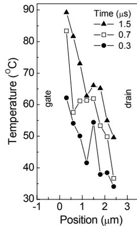
FIGURE 4: Temperature profile as a function of time in the gate-drain opening of an AlGaIn/GaN HFET on a SiC substrate (source-drain opening of 7.5  $\mu\text{m}$ , 2  $\mu\text{m}$  long gate), with the device operated with 2  $\mu\text{s}$  long 30 V (58 mA) square drain pulses at zero source-gate bias, 50% duty cycle; device width is 100  $\mu\text{m}$ . Electrical pulses start at  $t = 0$  s. Time resolution of the measurements was 200 ns.
