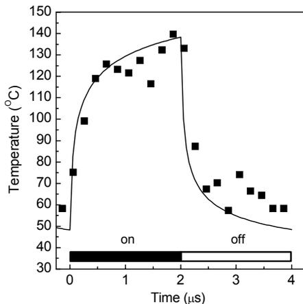
FIGURE 2: Temperature as function of time at the center of an ungated AlGaIn/GaN device on a SiC substrate with 5  $\mu\text{m}$  contact separation, grown on a SiC substrate, operated with 2  $\mu\text{s}$  long 20 V (165 mA) square bias pulses and a 50% duty cycle, together with simulation data; device width is 150  $\mu\text{m}$ . Time resolution of the measurement was 200 ns.
