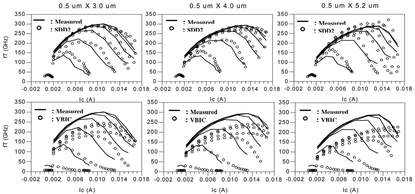
Figure 4: Measured  $f_T$  of three Vitesse VIP2 DHBT devices of different device sizes compared to results generated by Scalable SDD2 and VBIC model. ( $V_{ce}$ : 0 – 1.4 V,  $I_b$ : 20uA – 160 uA)
