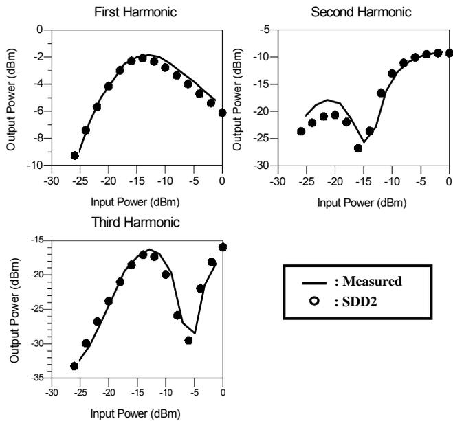
Figure 6: Measured and SDD2 modeled output of a  $0.5 \times 3.0 \mu m^2$  device with 2 GHz input tone swept from -25 dBm to 0 dBm
