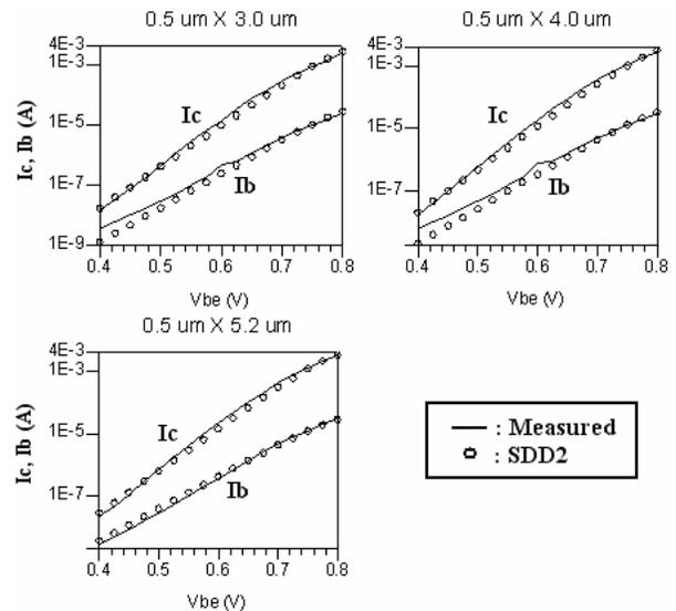
Figure 5: Measured and modeled forward Gummel data ( $I_c$  and  $I_b$ ) with respect to  $V_{be}$  as  $V_{cb}$  is held at zero volts
