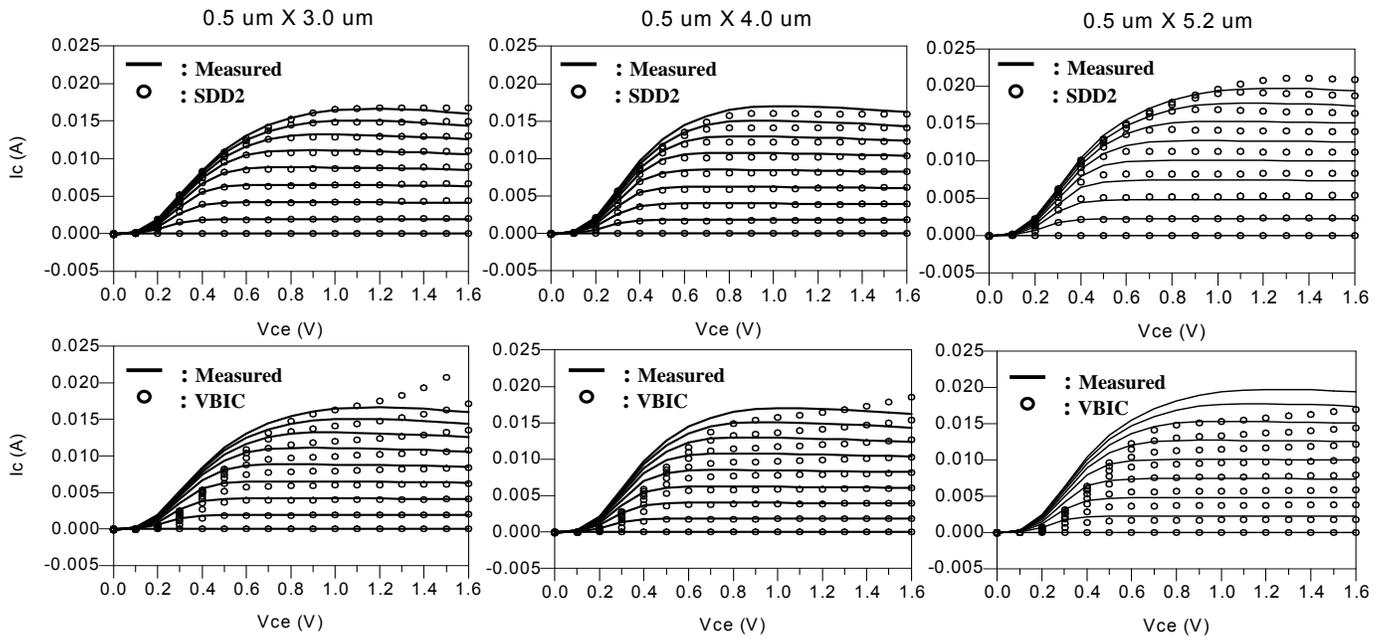
Figure 3: IV families of three measured Vitesse VIP2 DHBT devices of different size plotted with modeling results generated from both the Scalable SDD2 and VBIC model. (Vce: 0 – 1.6V, Ib: 0 – 160 uA)
