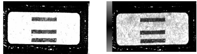
Figure 12: C-SAM figures revealing no change in die attach before (left) and after (right) temperature cycling.
